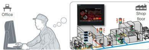
Figure 2: VNC server function helps achieve monitoring and maintenance from the office or other remote locations.
