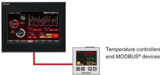
Figure 6: The addition of an RS-485 interface enables the connection of a wider range of devices such as temperature controllers and MODBUS® peripherals.
