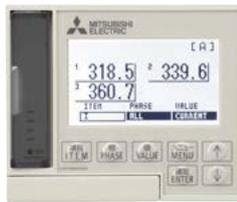
The conditions of **three phases are displayed in one window** and can be seen at a glance.
