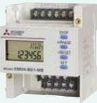
Using the built-in LCD screen, the energy consumption measured per unit can be displayed and the measurement value indicated. Since the RS-485 (MODBUS RTU) communication function is incorporated, when using the free data collection software, the present value of data being measured can be displayed on a PC and the CSV file acquired.
