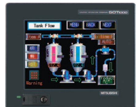
The GOT is a typical HMI
