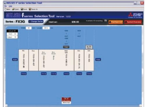
The selection tool provides all important information like power consumption, I/O point alignment and system size. A special page lists all the components in a table and provides the possibility to copy or print the information. Each configuration can be saved for machine ordering or documentation purposes. Please contact your local Mitsubishi Electric representative for more information.
