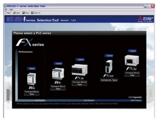
Then select the desired main unit type, different options for the power supply, number of I/O points and output format are available.
