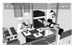
Advance checks of mechanical interference in 3D
