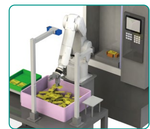
Picking from a large pallet (Fixed camera)
