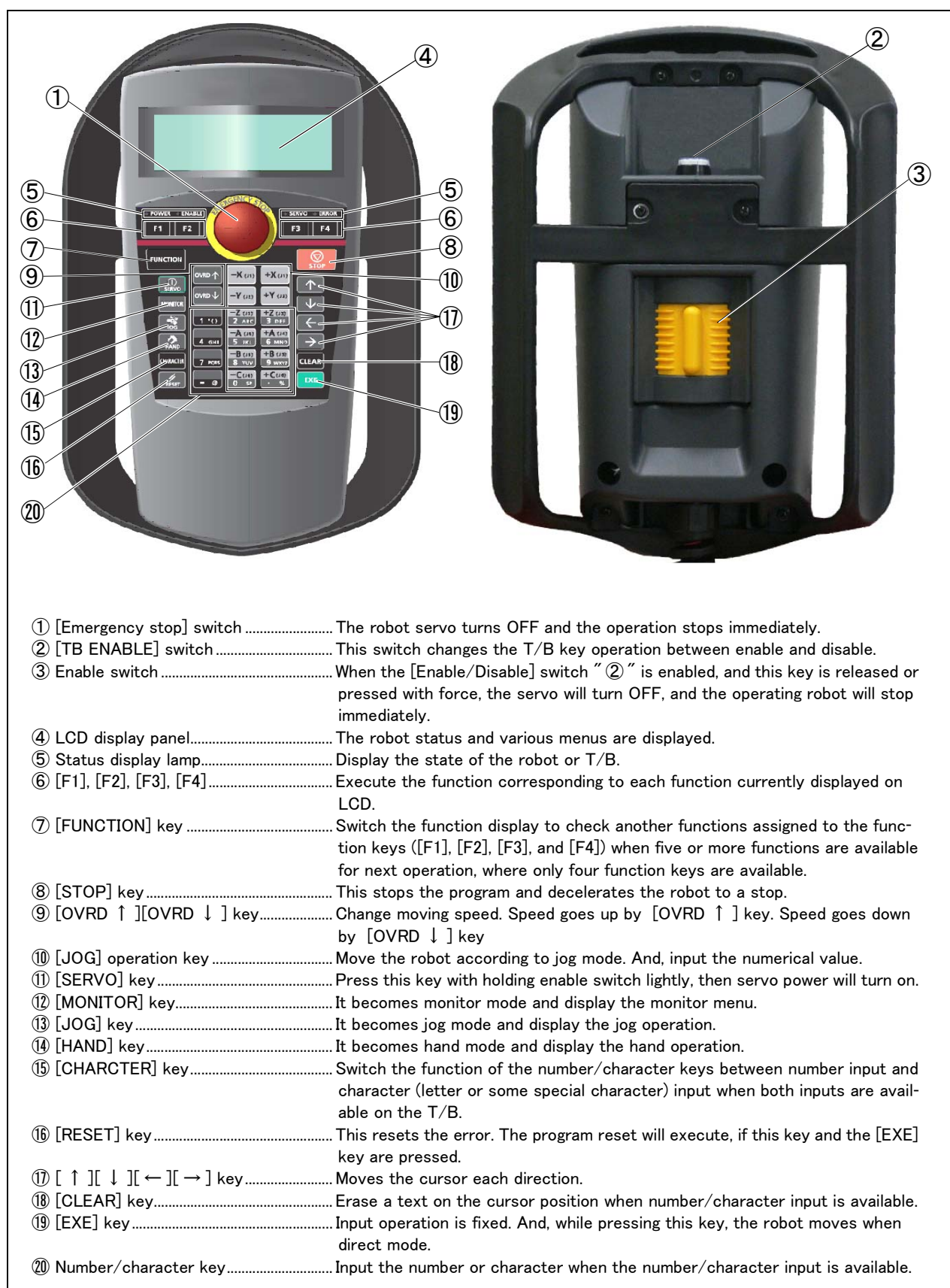
Fig.3-24 : Teaching pendant key layout and main functions
