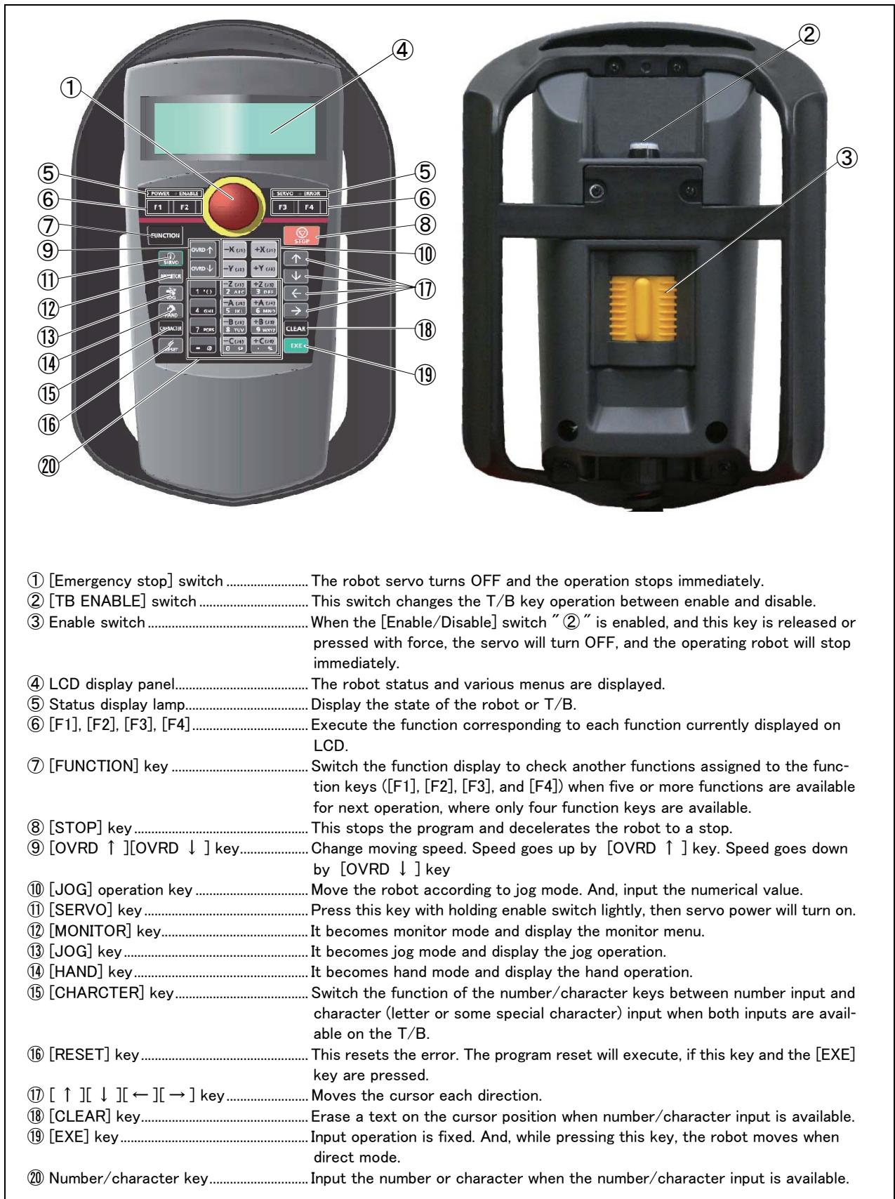
Fig.3-24 : Teaching pendant key layout and main functions
