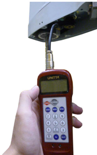
Fig.5-8 : Tension adjustment method of timing belt
