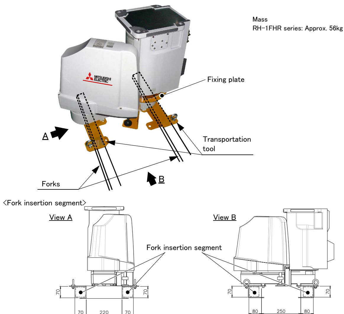
Fig.2-3 : Transportation of robot arm
