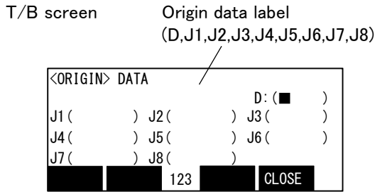
Fig.5-17 : Correspondence of origin data label and axis
