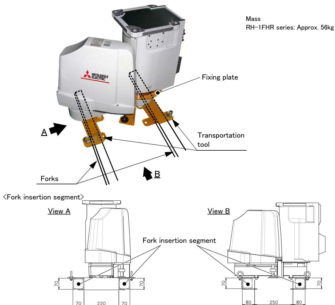
Fig.2-3 : Transportation of robot arm
