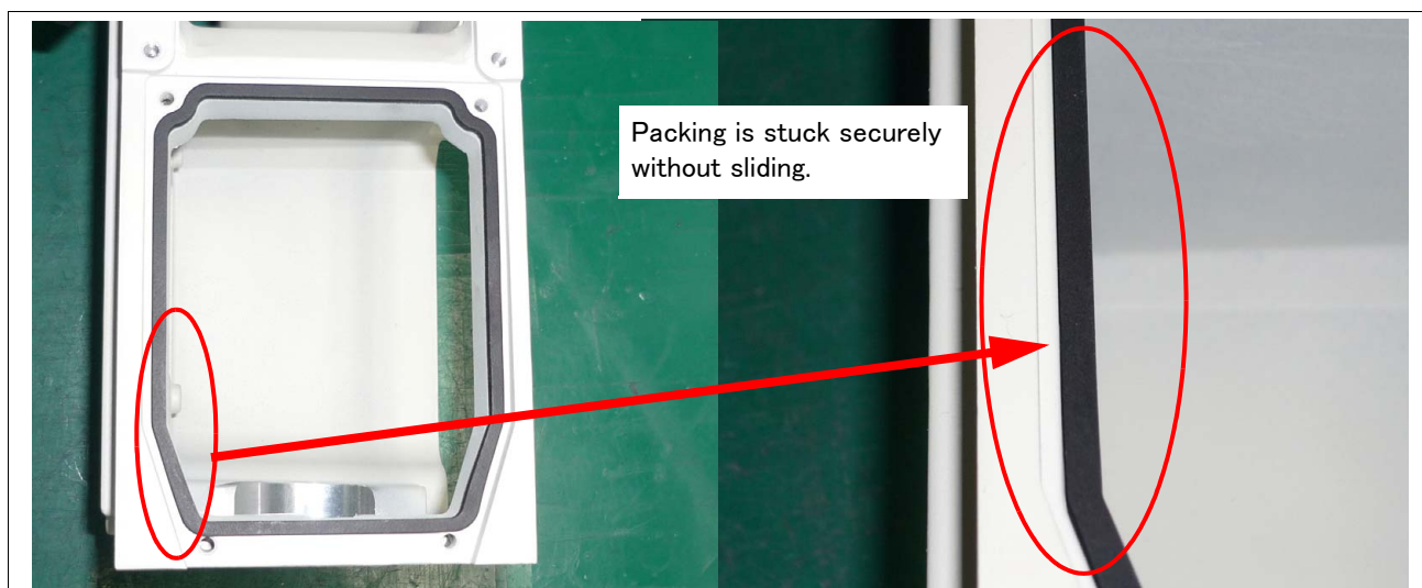
Fig.5-3 : Example of sticking packing (good example)
