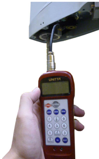
Fig.5-8 : Tension adjustment method of timing belt
