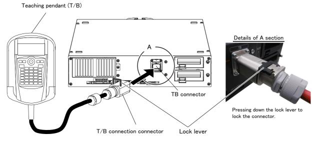
Fig. 2-12: Installing the T/B
