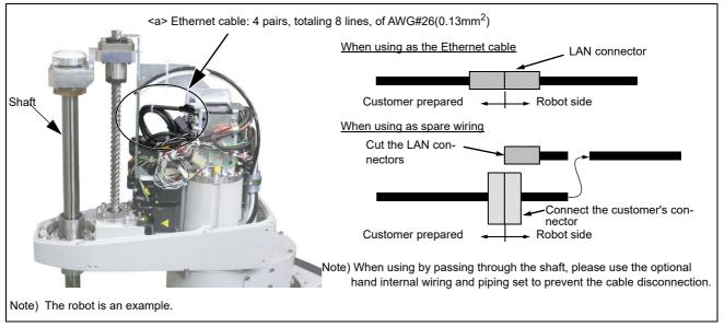
Fig.2-9: Pulling out the Ethernet cable
