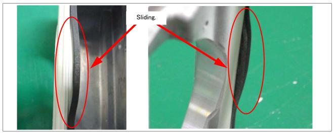
Fig.5-4 : Example of sticking packing (bad example)
