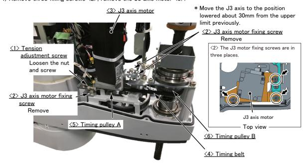
5) Remove the timing belt <4> from the timing pulley A <5>.
