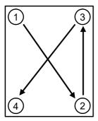
Fig.5-7: Example of order which tighten bolts
