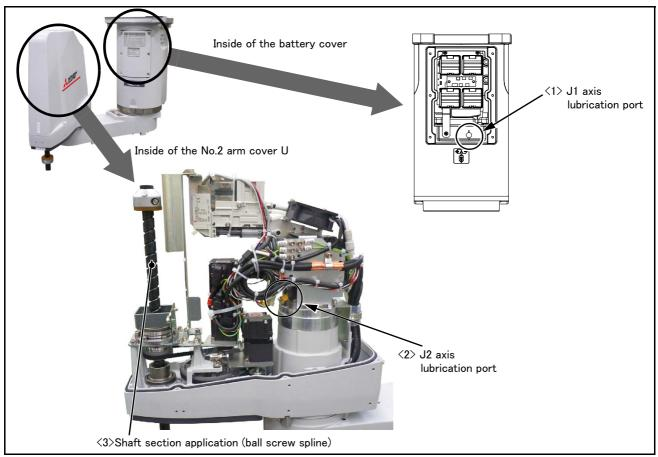
Fig.5-13: Lubrication positions
