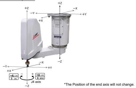
• When the [+C (J6)] keys are pressed, the J4-axis will rotate in the plus direction. When the [-C (J6)] keys are pressed, rotate in the minus direction.
