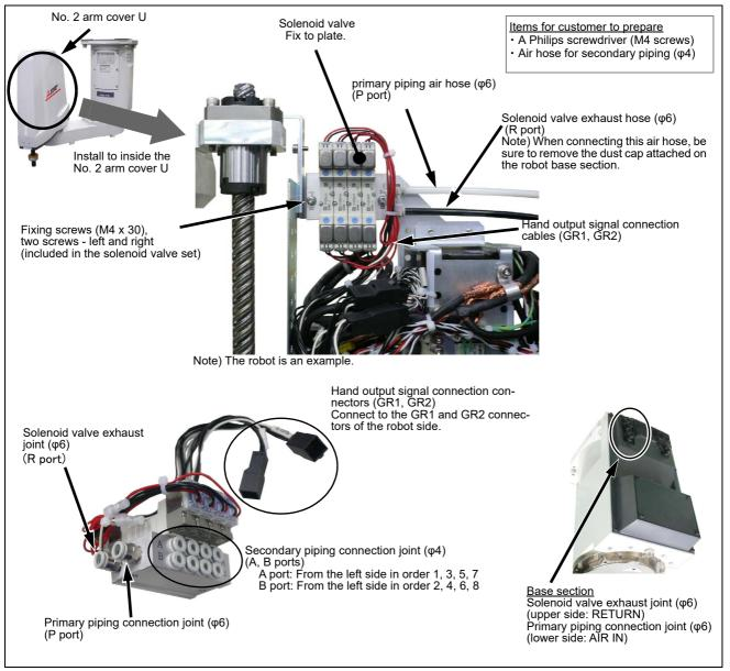
Fig.3-1: Solenoid valve installation procedures
