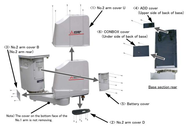
Fig.5-2: Installing/removing the cover
