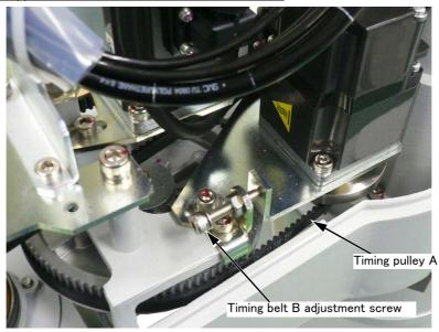
Fig.5-11: Inspecting the J4 axis timing belt(RH-/6FRH/12FRH/20FRH)
