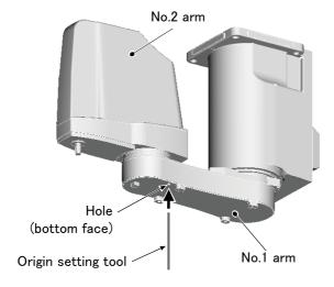
2) Move the J2 axis slowly with both hands to the position around  $\pm 0^{\circ}$ . And align the pinholes of the No. 1 and No. 2 arms, feed through the origin jig into the pinholes and fasten.
