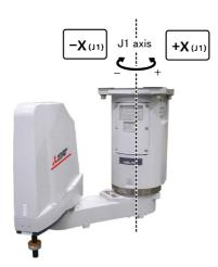
• When the [+X (J1)] keys are pressed, the J1 axis will rotate in the plus direction. When the [-X (J1)] keys are pressed, rotate in the minus direction.
