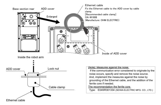
Fig.2-10: Pull out the Ethernet cable (Base side)
