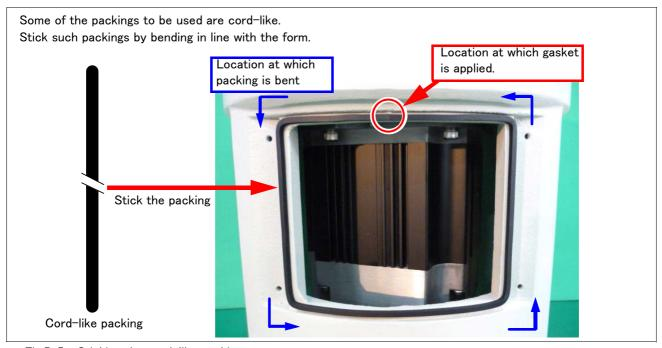
Fig.5-5: Sticking the cord-like packing
