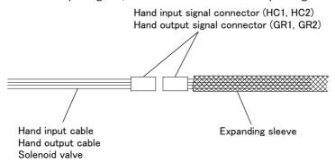
2) Connect the HC1 and HC2 connectors for the hand input signals and the GR1 and GR2 connectors for the hand output signals, and cover the joint part with the expanding sleeve.
