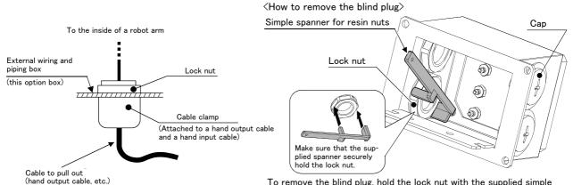
To remove the blind plug, hold the lock nut with the supplied simple spanner for resin nuts, and loosen the cap with a screwdriver. The supplied simple spanner is used when attaching a cable clamp the same way.
