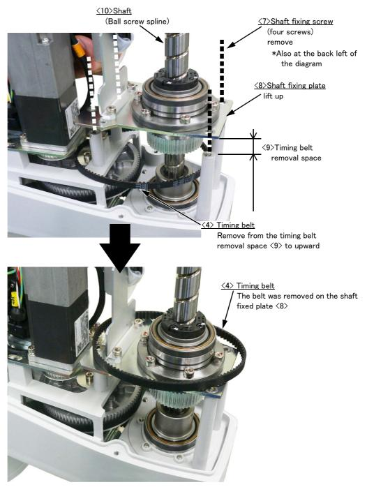
7) Remove the timing belt <4> from the top of the shaft If using the optional hand internal wiring and piping set, temporarily remove the hand input cable connector <11> and air hoses <12> of solenoid valve side. And remove the timing belt to upward.
