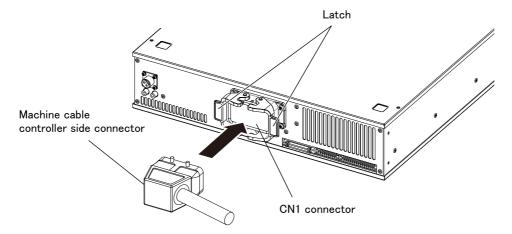
Fig.2-8: Connecting with the controller
