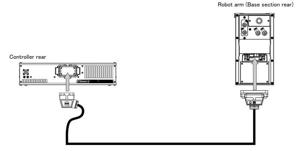
Fig.2-7: Connecting the machine cables
