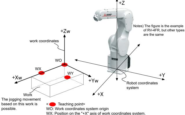
WY: Position at the side of "+Y" axis on the X-Y plane of work coordinates system.
