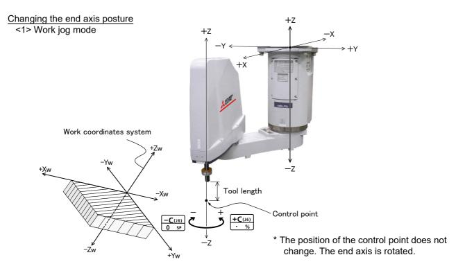
• When the [+C (J6)] keys are pressed, the Z axis will rotate in the plus direction of the XYZ coordinate system. When the [-C (J6)] keys are pressed, rotate in the minus direction.
