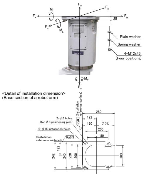
Fig.2-4: Installation dimensions
