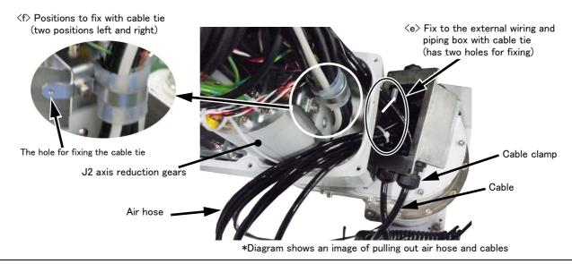
Fig.3-6: External Wiring and Piping Box
