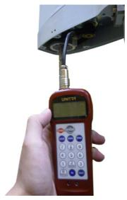
Fig.5-8: Tension adjustment method of timing belt
