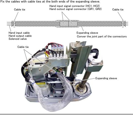
3) Arrange the expanding sleeve in a ring-like shape and fix it with a cable tie.
