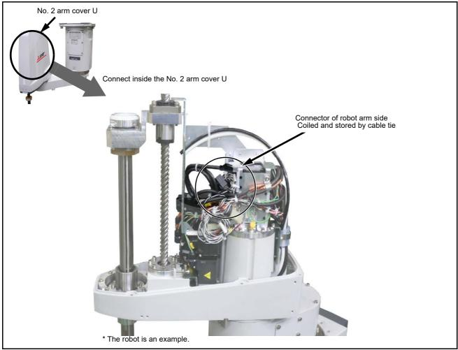
Fig.3-3: Installing the hand output cable
