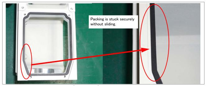
Fig.5-3: Example of sticking packing (good example)
