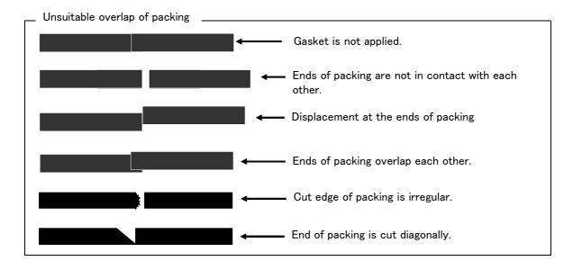
Fig.5-6: Examples of packing overlaps
