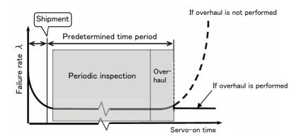
Fig.5-15: Periodic inspection/overhaul periods
