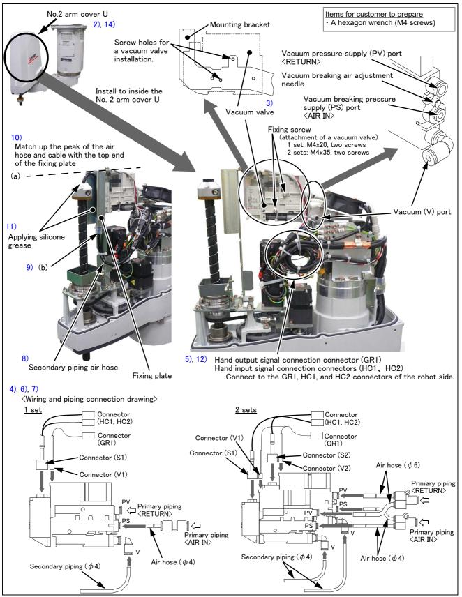
Fig.3-8: Vacuum valve installation procedures
