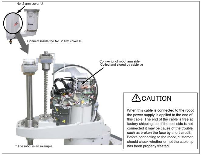
Fig.3-2: Installing the hand input cable
