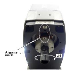
8) Hold the J4 axis with your hand and rotate it slowly to match the alignment marks. Move the J4 axis with maintaining the condition that the releasing brake of the J3 axis and the J3 axis contact to the mechanical stopper. Note) If the J3 axis has slid, move the J3 axis against the mechanical stopper, and contact again.
