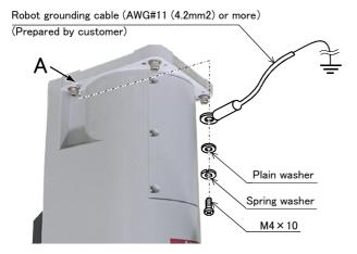
Fig.2-6: Connecting the grounding cable
