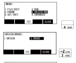
2) Press the [4] key on the menu screen, and display the Origin/Break selection screen.
