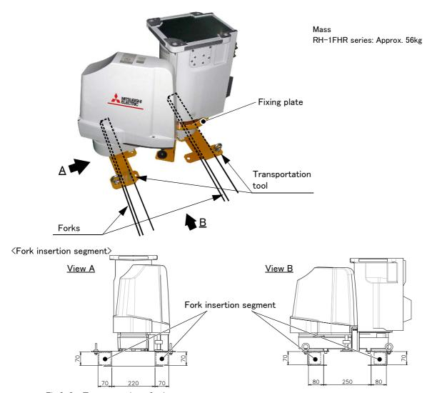
Fig.2-3: Transportation of robot arm
