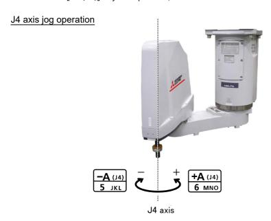
• When the [+A (J4)] keys are pressed, the J4 axis will rotate in the plus direction. When the [-A (J4)] keys are pressed, rotate in the minus direction.
