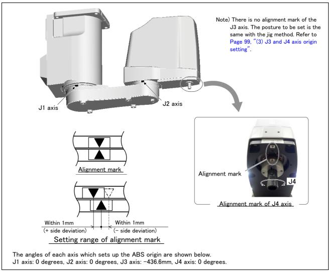
Fig.5-19: ABS mark attachment positions
