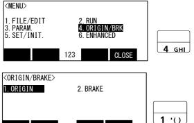
1) Press the [4] key on the menu screen, and display the ORIGIN/BRAKE screen.
