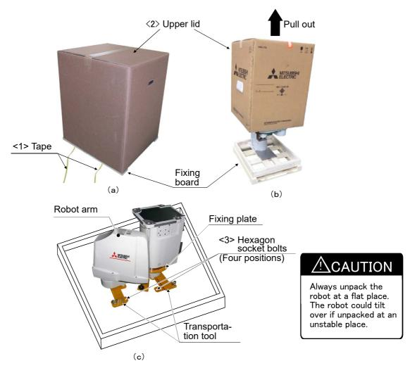
Fig.2-1: Unpacking the robot arm
