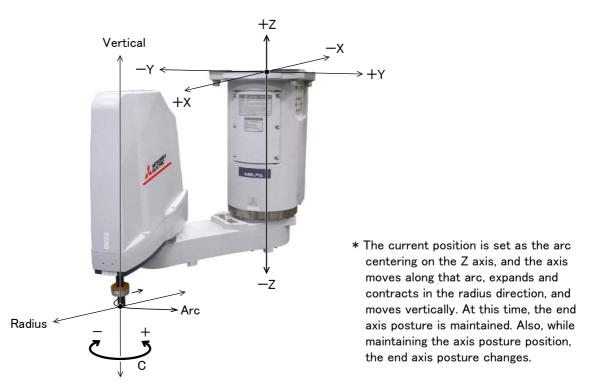
Fig.2-17: CYLINDER jog operation
