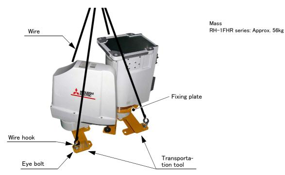
Fig.2-2: Transportation of robot arm
