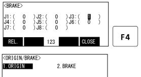
9) Detach the [F1] key and work the brake. Press the [F4] key and return to the origin / brake screen.
