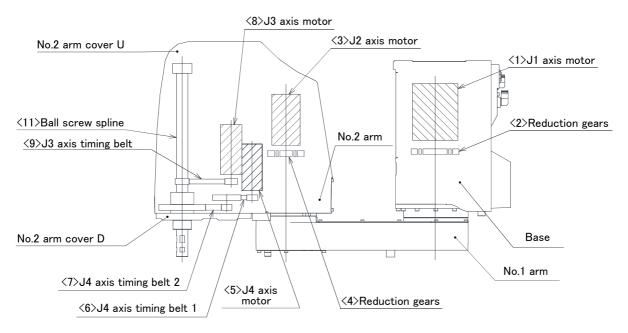
Fig.5-1: Outline structure drawing of robot arm
