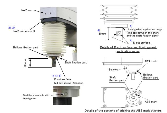
Fig.5-12: Replace the bellows (option)
