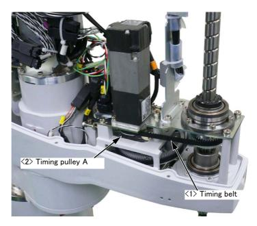
Fig.5-10 : Inspecting the J3 axis timing belt
