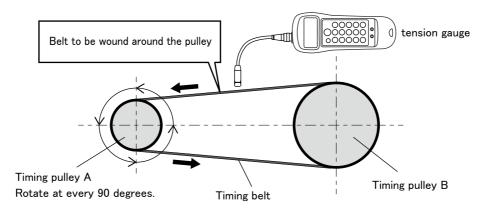
Fig.5-9: Timing belt tension measurement
