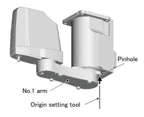
2) Move the J1 axis slowly toward the front using both hands. Align the pinhole of the No.1 arm and the pinhole at the base section, feed through the origin jig into the pinholes and fasten.
