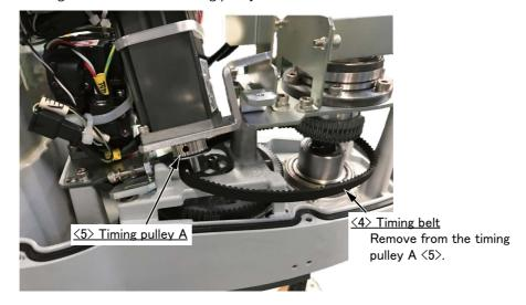
6) Remove the timing belt <4> from the shaft to upward. Remove the fixing screw  $\langle 7 \rangle$  of shaft fixing plates and lift up the shaft fixing plate  $\langle 8 \rangle$ . When using the optional hand internal wiring and piping set remove the fixing screws fixed to the top. Remove the timing belt <4> from the timing belt removal space <9> created under the shaft fixing plate <8> by lift up.
