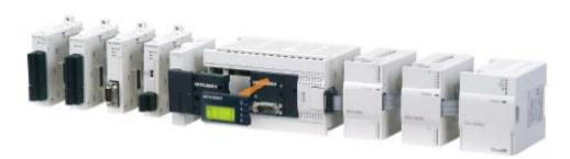
Mitsubishi's migration path allows users to extract a programme from a 25 year old PLC (e.g. F Series) and easily convert the code for use in the very latest FX3 generation PLCs. Also near-identical footprints of next generation PLCs mean that there are no physical problems to replacing old technology with new.
