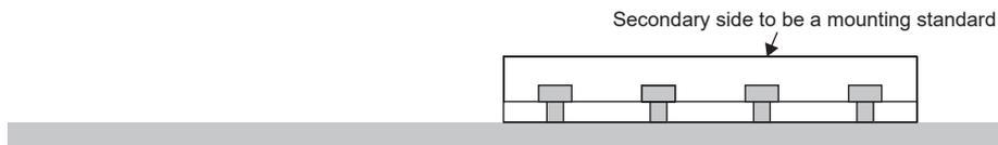
2. Set the next secondary side on the mounting face and use bolts to temporarily fix it into place.
