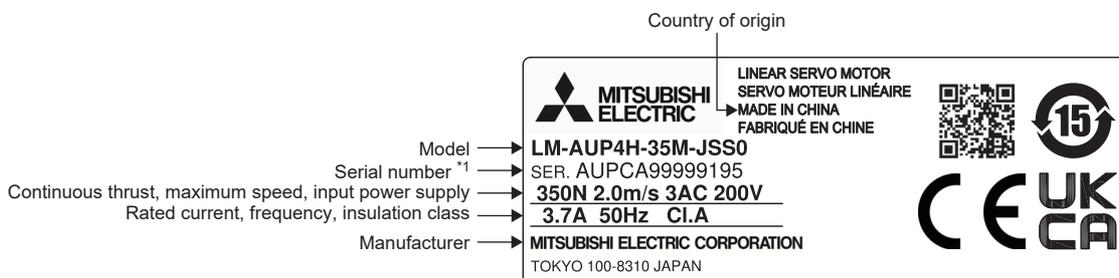
\*1 The date of manufacture of the primary side of the linear servo motor are indicated in the serial number on the rating plate. For the date of manufacture, the last two digits of the year and the month in numerical format [1 to 9, X (10), Y (11), and Z (12)] are displayed.
