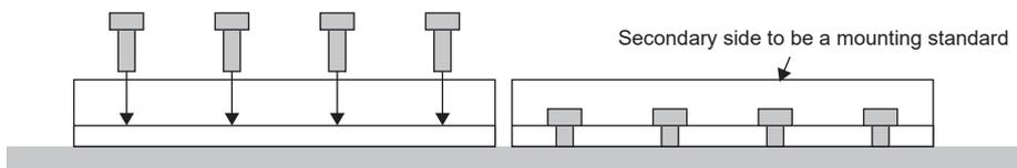
3. Press the added secondary side toward the secondary side that is being used as the mounting standard.
