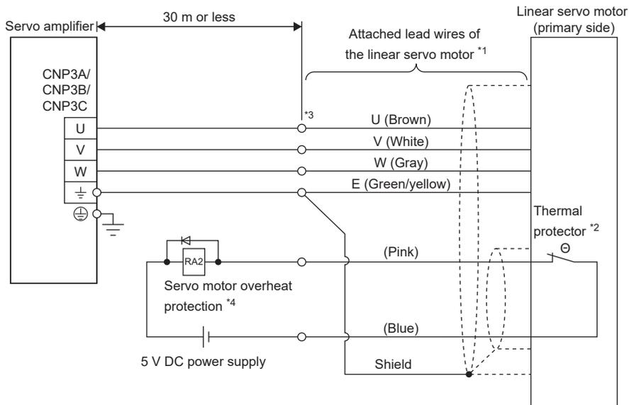
\*1 The signal names are not attached on the lead wires. Use the color of the wire to determine which signal it is for.
