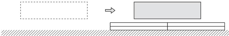
4. Mount the rest of the secondary sides. Confirm that the primary and secondary sides are not touching each other.
