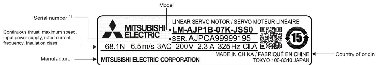
\*1 The date of manufacture of the primary side of the linear servo motor are indicated in the serial number on the rating plate. For the date of manufacture, the last two digits of the year and the month in numerical format [1 to 9, X (10), Y (11), and Z (12)] are displayed.
