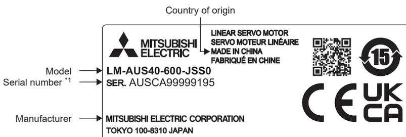
\*1 The date of manufacture of the secondary side of the linear servo motor are indicated in the serial number on the rating plate. For the date of manufacture, the last two digits of the year and the month in numerical format [1 to 9, X (10), Y (11), and Z (12)] are displayed. For January 2012, the serial number would be "SER. \_\_\_\_\_ 121".
