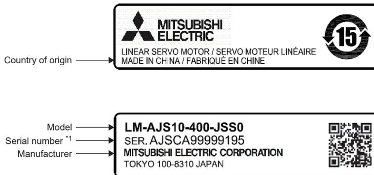
\*1 The date of manufacture of the secondary side of the linear servo motor are indicated in the serial number on the rating plate. For the date of manufacture, the last two digits of the year and the month in numerical format [1 to 9, X (10), Y (11), and Z (12)] are displayed. For January 2012, the serial number would be "SER. \_\_\_\_\_ 121".
