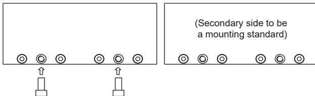
3. Leave a gap of 0.5 mm between the temporarily fixed secondary side and the mounting-standard secondary side.
