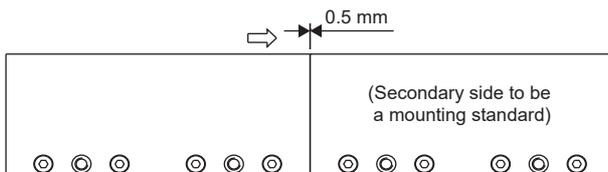
4. Use bolts to securely fix the added secondary side into place.
