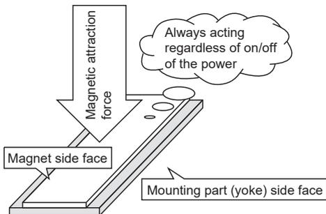
The magnetic fluxes generated by the permanent magnet are dispersed into the air from the magnet face side (the side facing the primary side), and most of said fluxes do not leak to the mounting part (yoke) surface side due to its structure.
