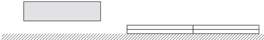
3. Move the primary side over the mounted secondary side. Confirm that the primary and secondary sides are not touching each other.
