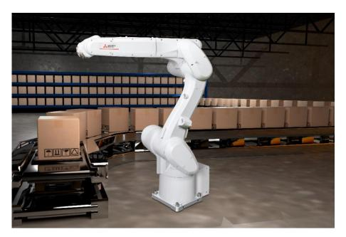
[Source: Mitsubishi Electric Europe] Image caption: Mitsubishi Electric's latest MELFA RV-12CRL vertical articulated robot supports industrial automation pick-and-place applications with a 1,504 mm reach and 12 kg payload capacity.
