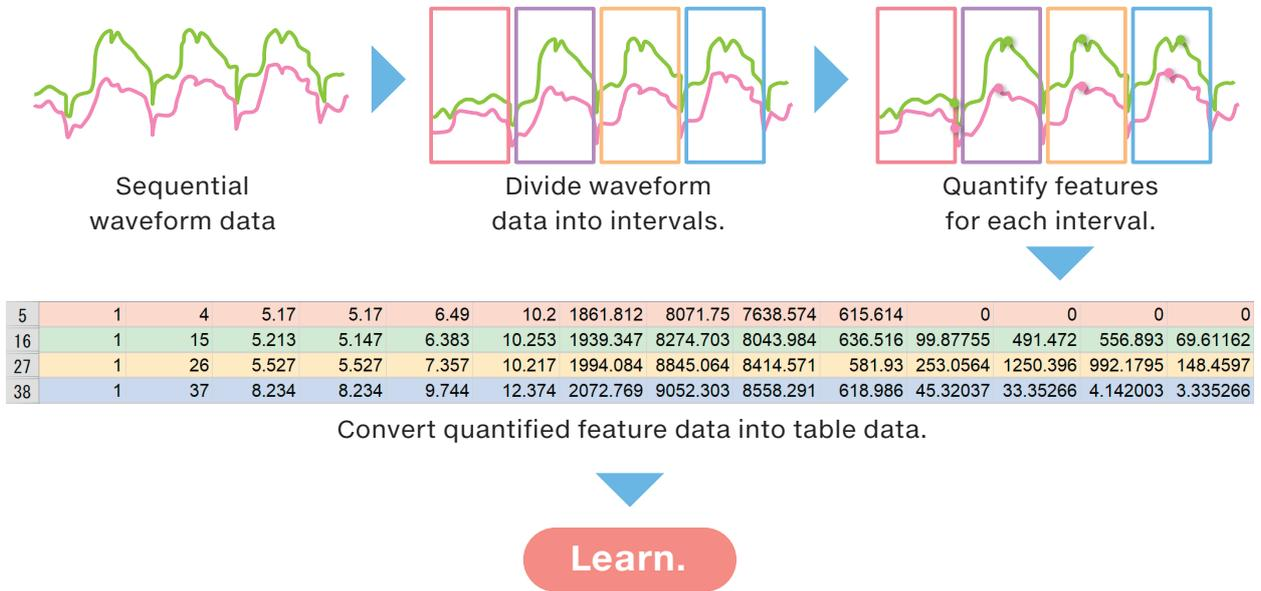
In “Variable indicating interval start”, specify the marker that AutoML function will use to divide the intervals.
