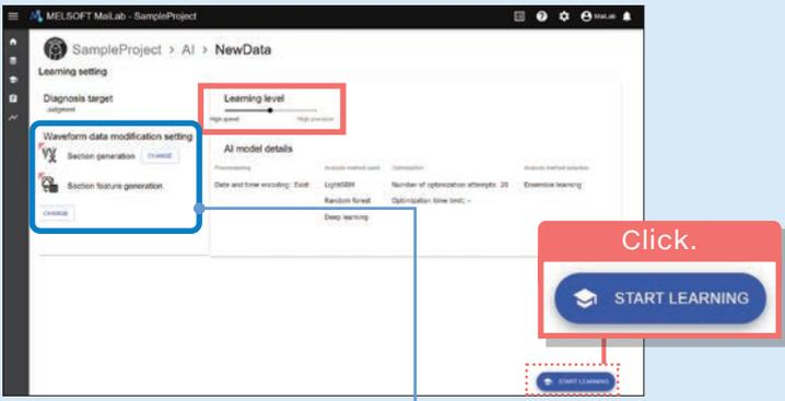
The waveform data set will be displayed, and the detailed settings for interval dividing can be set. When interval division is performed using the contents of the simple settings in Step 1 7, setting (changing) is not necessary. When performing detailed settings, refer to “5.2.3 Feature quantity engineering: (2) Taking a specific part of the data and extracting features”.
