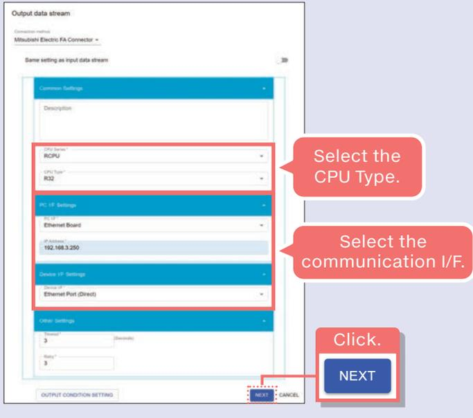
Set the model information and communication method for the write target, and click the “NEXT” button.
