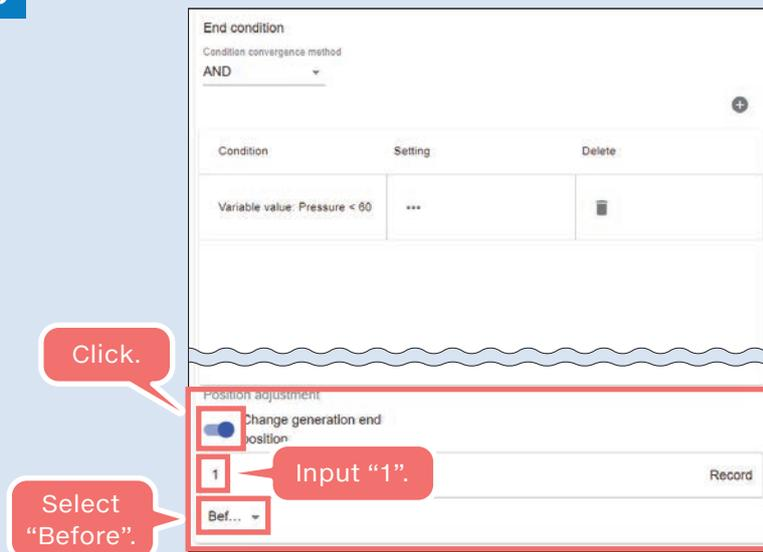
With the condition "Pressure < 60", the portion until the first record where pressure is below 60 will be the cut out target.
