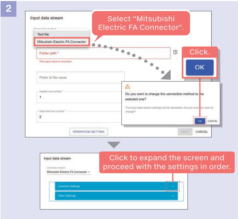
The input data stream dialog will appear. Select “Mitsubishi Electric FA Connector” for Connection method and click the “OK” button in the change confirmation dialog.
