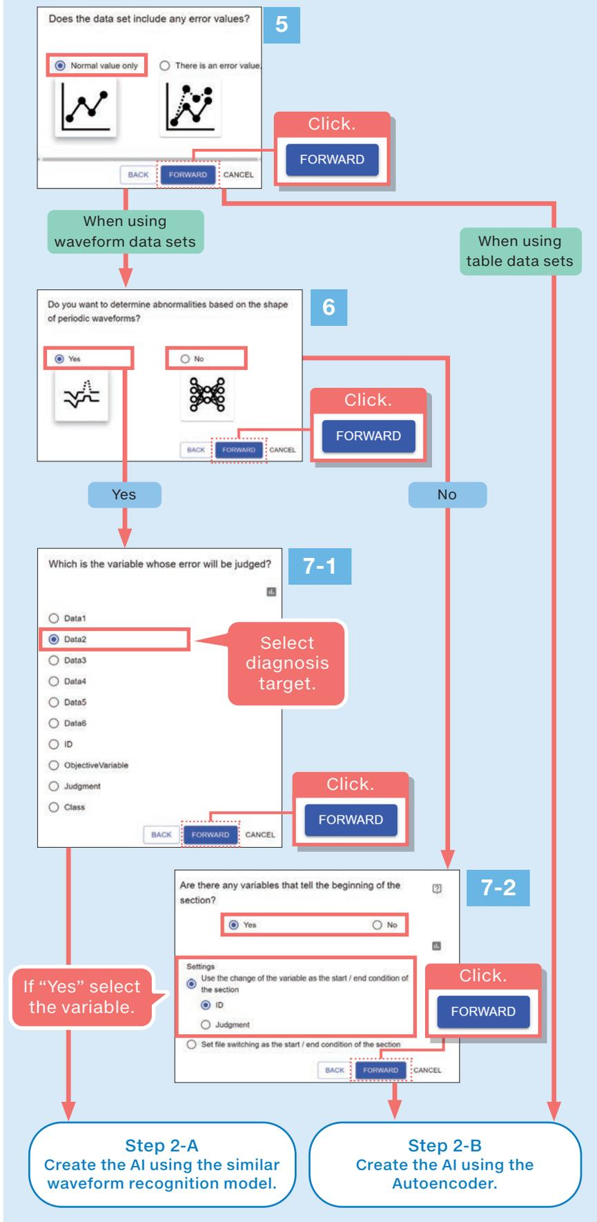
**5** Select “Normal value only” and click the “FORWARD” button. When using table data sets, interactive ends here.
