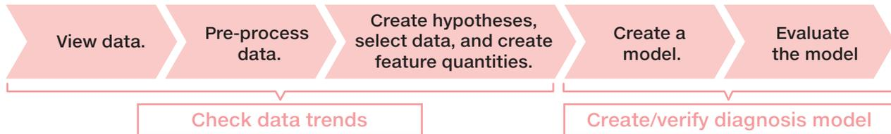
The 5 steps above are the general flow of offline analysis, in which collected data are analyzed and a model for solving issues is created. The above steps are not necessarily followed in one direction from left to right. In many cases there is a lot of going back and forth between steps.
