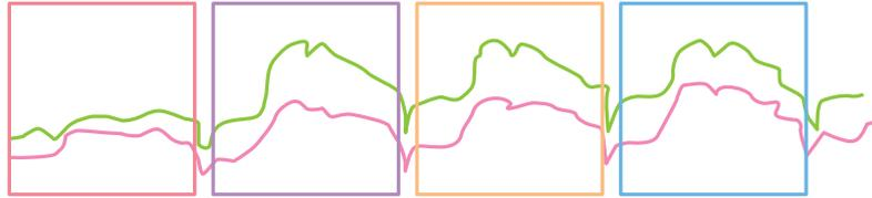
\* Interval: For waveform data with repeated patterns, 1 segment of the waveform data divided by pattern is called an "interval" in MaiLab. In addition, the length of an interval is called "interval length".
