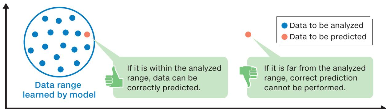
For example, when predicting a certain data, if the data to be predicted is within the range of data learned by the model in advance as shown in the above diagram, data can be predicted with high accuracy. However, for data which is far away from the analyzed data range, high prediction accuracy cannot be expected.
