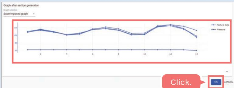
After interval creation, confirm that the interval which exceeds 60 was cut out, and click the “OK” button.
