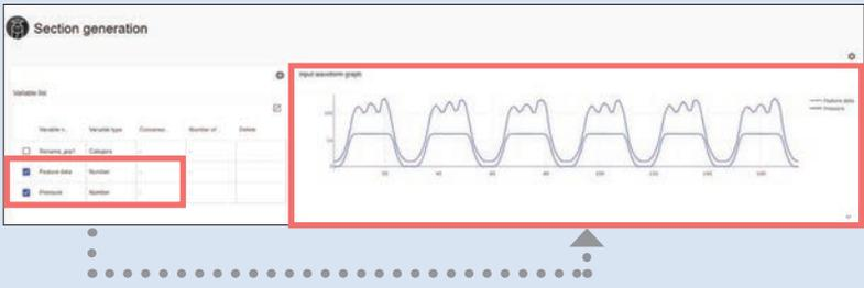
When the variable for checking the interval is selected, the input waveform graph for the selected variable will be shown. In this example, the feature data and pressure variables are used.
