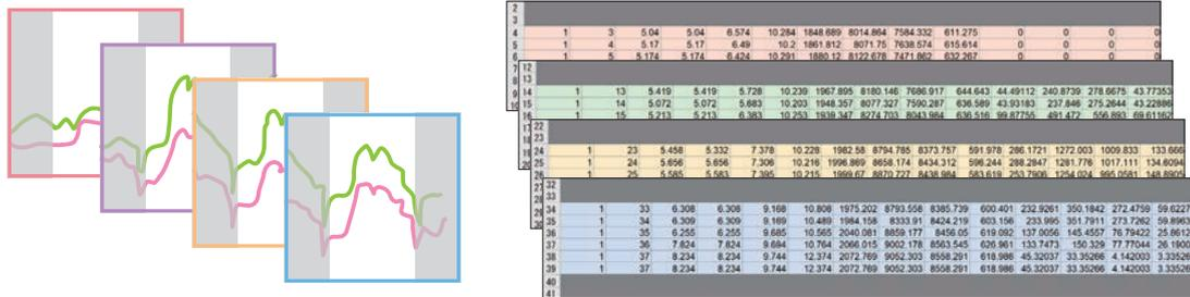
Waveform data for each interval are cut into smaller intervals.
