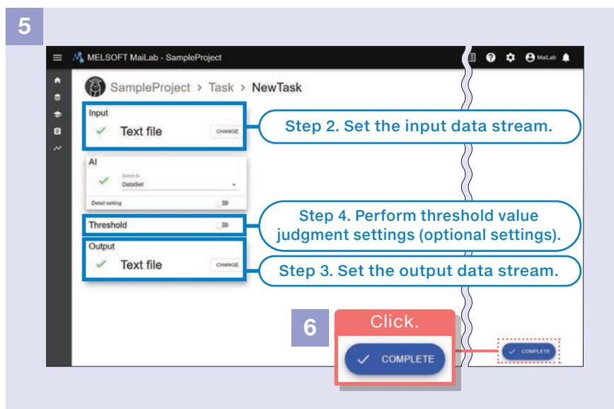
5 Proceed to the parameter setting dialog for each process of the simple task and set the parameters for each process. (Details are explained in Step 2 and later.)
