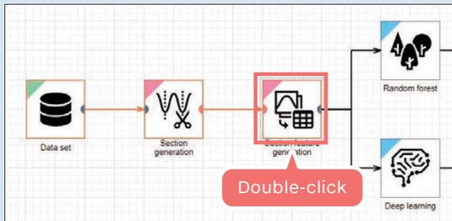
Double-click on the “Section feature generation” block to open the properties.
