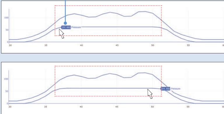
The graph will be enlarged. On the graph, check the value of the range where pressure is stable.
