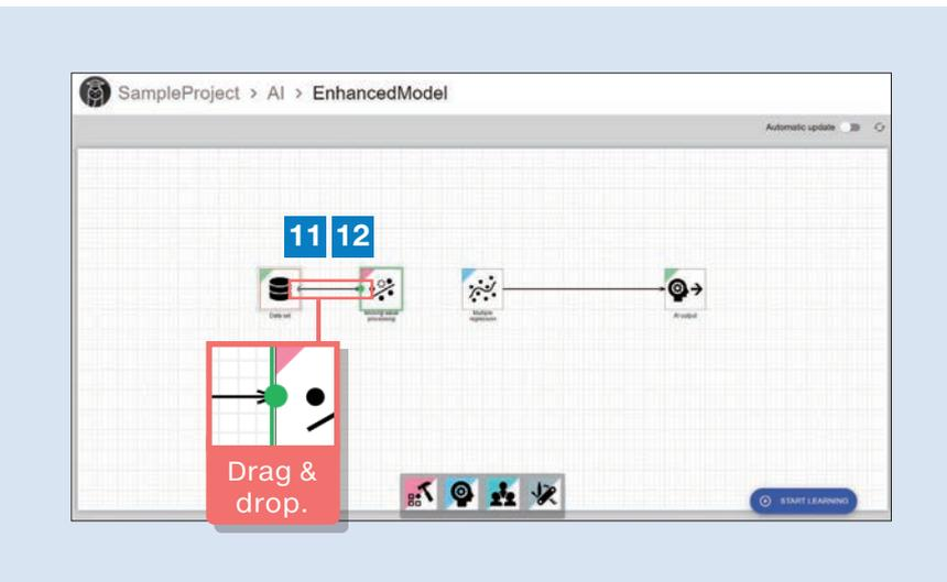
11 Drag it to the left edge of the block (on the downstream side of the data) that you want to connect to. An arrow connector following the pointer will appear.
