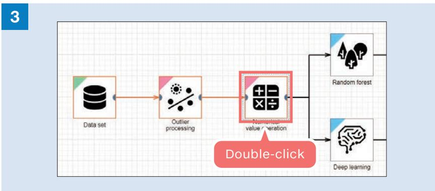
Double-click on the Numerical value operation block to open the properties.
