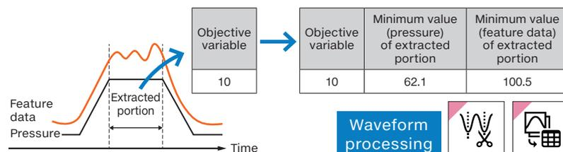
The portion where a value is constant and stable as in the above example is often linked to deterioration of mechanical systems.
