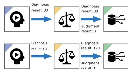
It can be utilized for performing threshold value judgment on diagnosis results (estimation value) and performing OK/NG (0/1) feedback to the PLC, etc.
