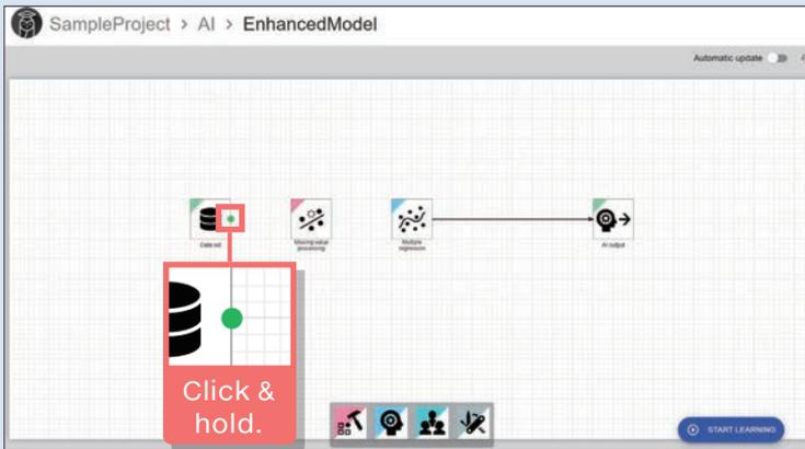
When the pointer is placed over the upstream block of data, a ● will appear on the right edge of the block. Click & hold the ●.
