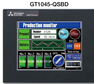
4.7 inch Screen size: 4.7 inch Resolution: 320 × 240 Display color: 256 colors
