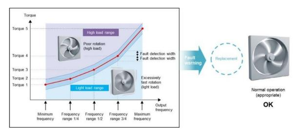
Preventive maintenance, often supported by features on inverters, can support early notification of potential abnormalities such as equipment failure. [Source: Mitsubishi Electric Corporation, Japan]
