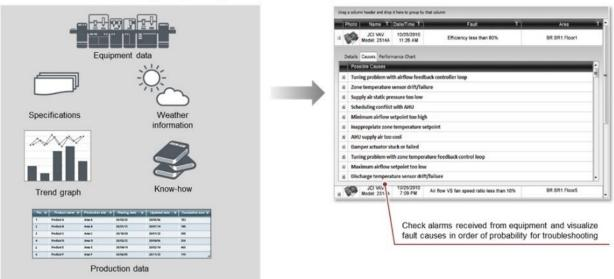
SCADA systems can be used to list-up potential fault causes in order of probability to make troubleshooting tasks easier - this example is from a GENESIS64 solution. [Source: Mitsubishi Electric Corporation, Japan]
