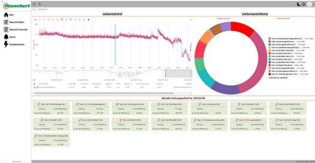
Pic 2: Implemented energy monitoring tool: The factory and specific buildings energy consumption overview.
