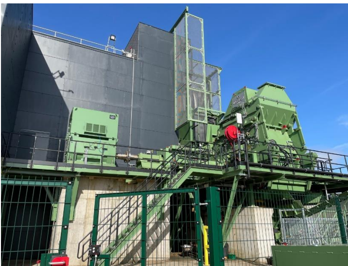
Image 1: With 3,000 hp, the LINDEMANN ZZ Power shredder is one of
