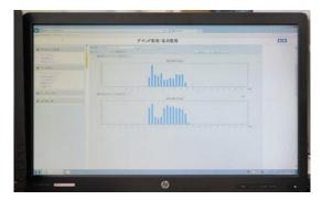
Image 7: This screen for monitoring the real-time electricity demand helps to efficiently control power consumption in the factory to avoid exceeding the contract demand level.
