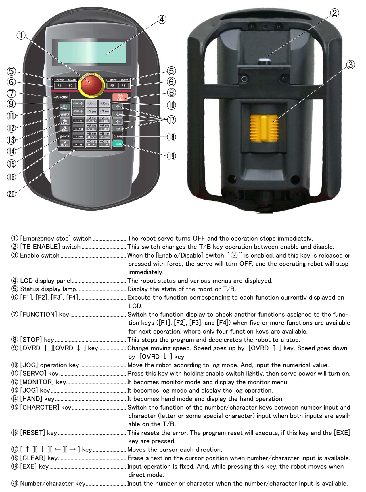
Fig.3-24 : Teaching pendant key layout and main functions
