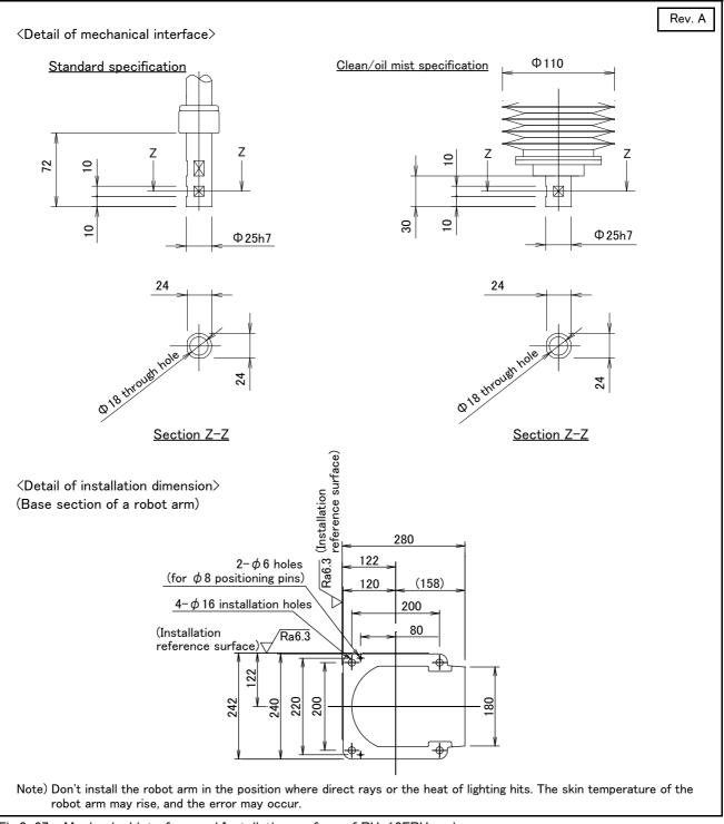
Fig.2-67 : Mechanical interface and Installation surface of RH-12FRH series
