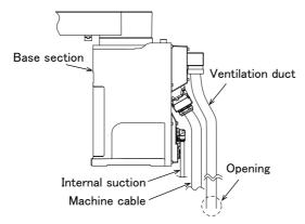
Fig.2-16 : Installation of Ventilation Duct
