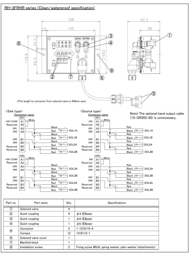
Fig.2-89 : Outline dimensional drawing (RH-3FRHR series: Clean/waterproof specification)
