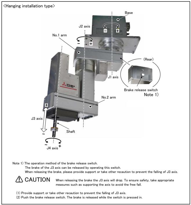
Fig.2-18 : Names of each part of the robot (Hanging installation type)
