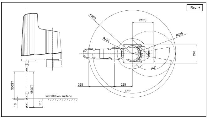
Fig.2-44 : Operating range diagram of RH-12FRH55xx
