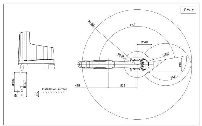
Fig.2--58 : Operating range diagram of RH-20FRH100xx
