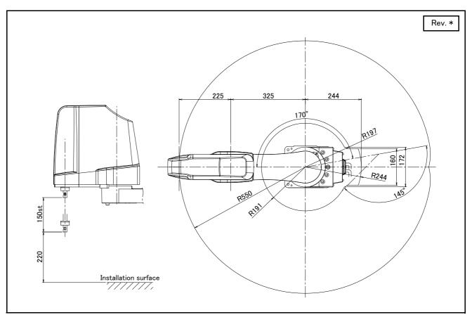
Fig.2-24 : Operating range diagram of RH-3FRH5515
