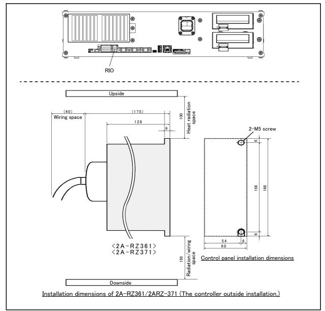
Fig.3-38 : Installing the parallel I/O unit
