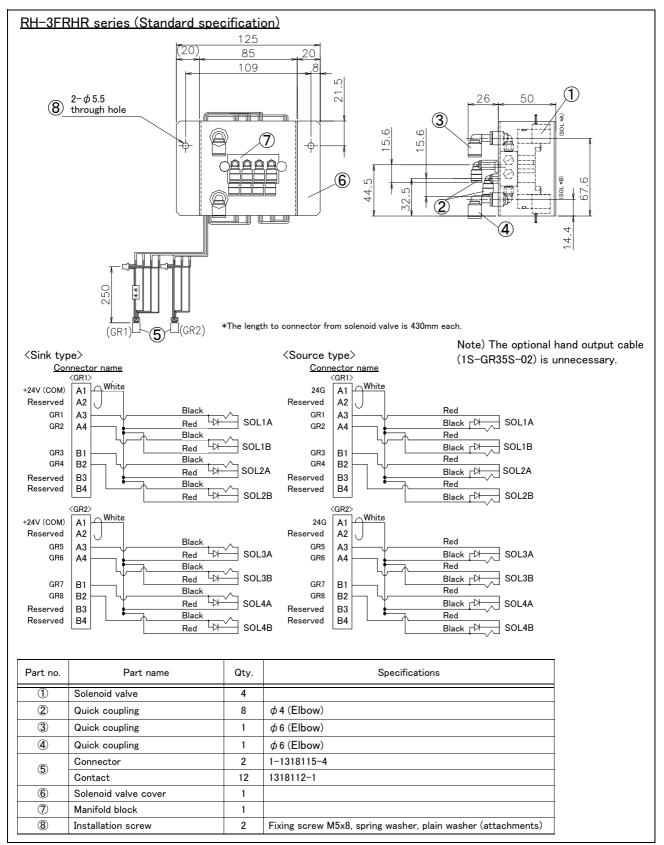
Fig.2-88 : Outline dimensional drawing (RH-3FRHR series: Standard specification)
