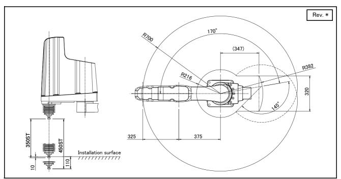
Fig.2-52 : Operating range diagram of RH-12FRH70xxC/M
