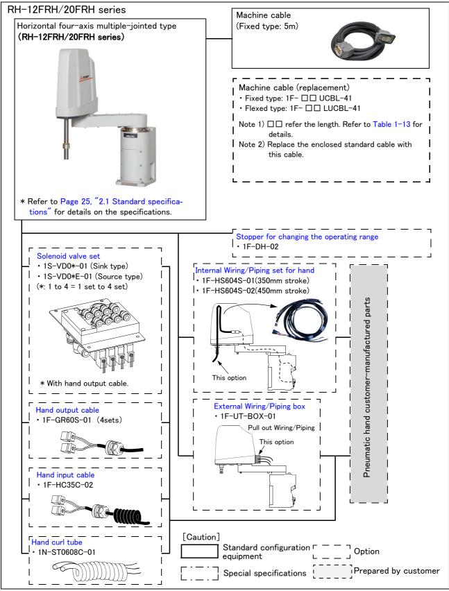
Fig.1-3 : Structural equipment (RH-12FRH/20FRH series)
