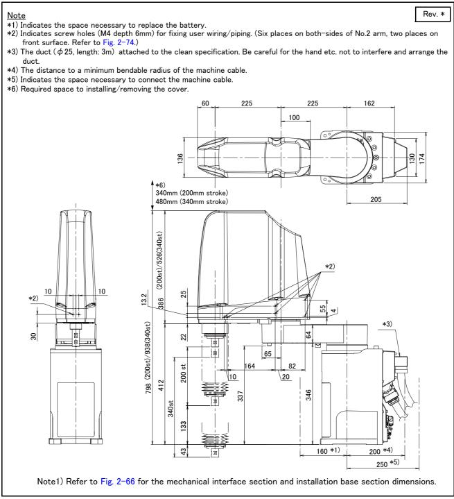
Fig.2-39 : Outside dimensions of RH-6FRH45xxC/M
