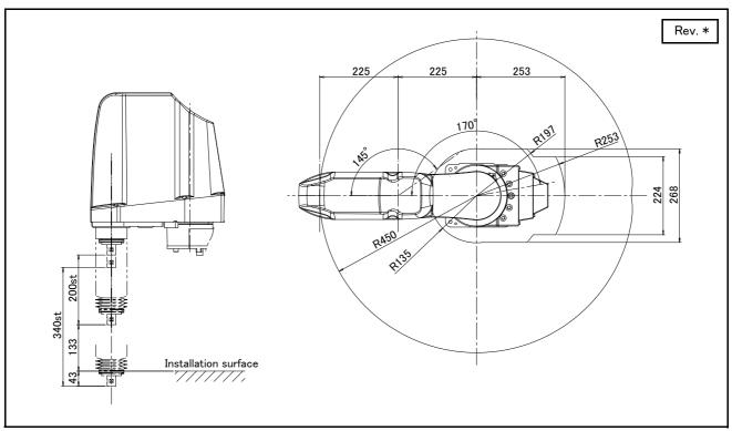
Fig.2-40 : Operating range diagram of RH-6FRH45xxC/M
