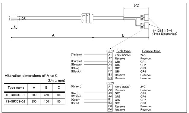
Fig.2-92 : Outline dimensional drawing and pin assignment
