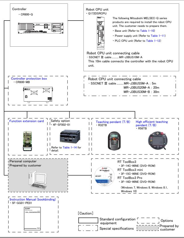
Fig.1-7 : Structural equipment (CR800-Q)
