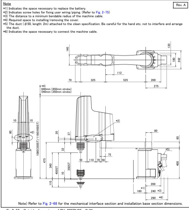
Fig.2-59 : Outside dimensions of RH-20FRH85xxC/M
