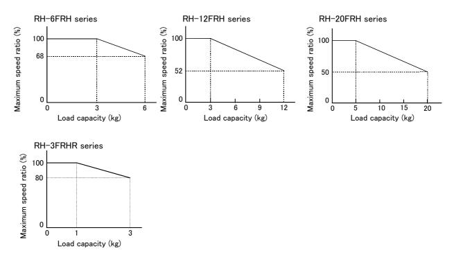
Fig.2-8 : Automatic compensation of speed
