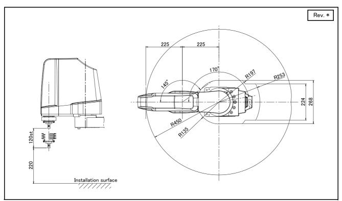
Fig.2-28 : Operating range diagram of RH-3FRH4512C
