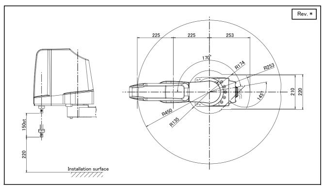
Fig.2-22 : Operating range diagram of RH-3FRH4515
