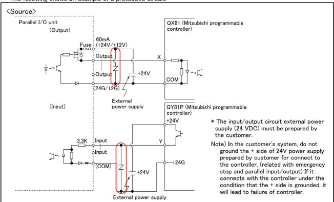
The following shows an example of a protective circuit.
