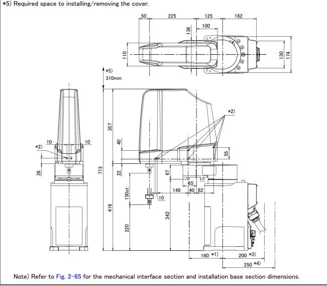
Fig.2-19 : Outside dimensions of RH-3FRH3515
