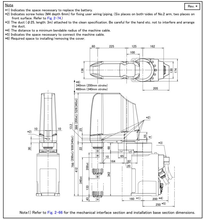
Fig.2-37 : Outside dimensions of RH-6FRH35xxC/M
