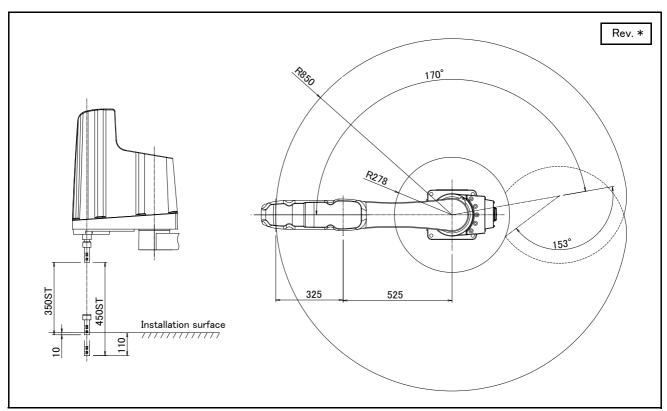
Fig.2-48 : Operating range diagram of RH-12FRH85xx
