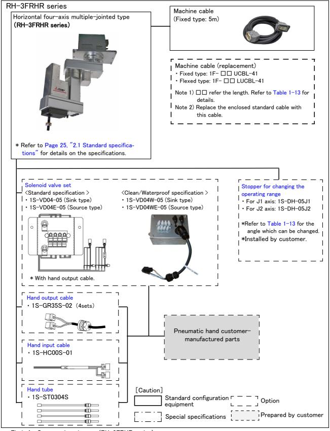
Fig.1-4 : Structural equipment (RH-3FRHR series)
