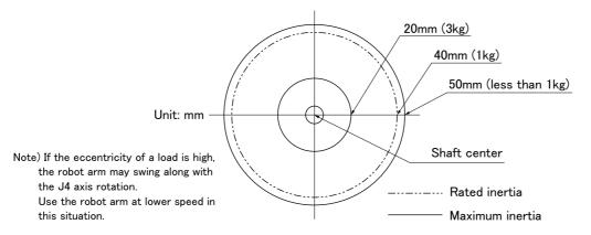
Fig.2-7 : Position of center of gravity for loads (for loads with comparatively small volume): RH-3FRHR series
