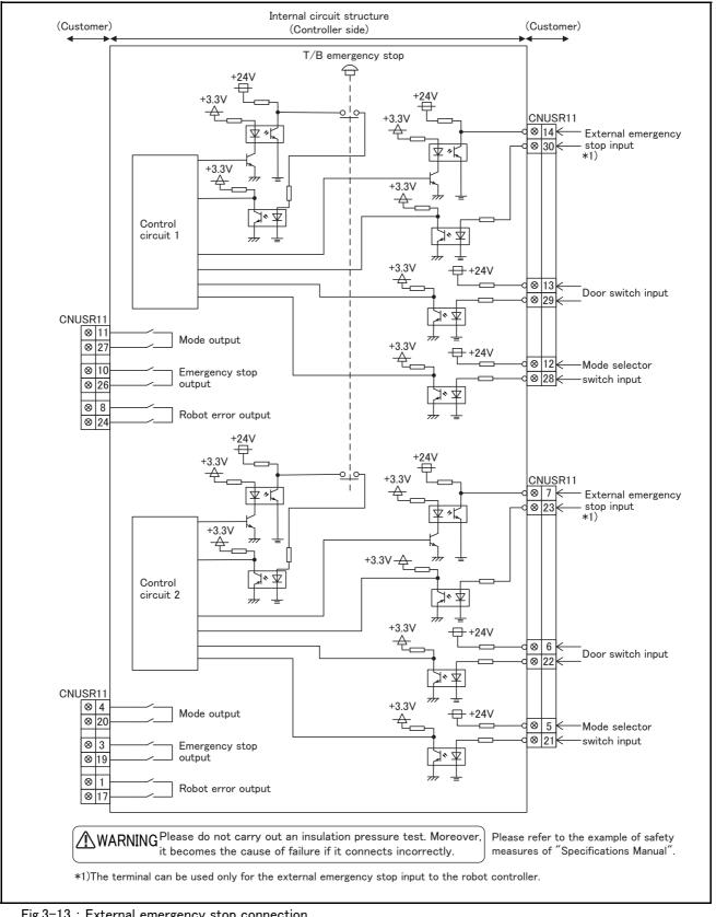
Fig.3-13 : External emergency stop connection
