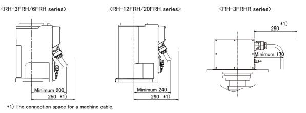
Fig.2-85 : Fixing the flexible cable
