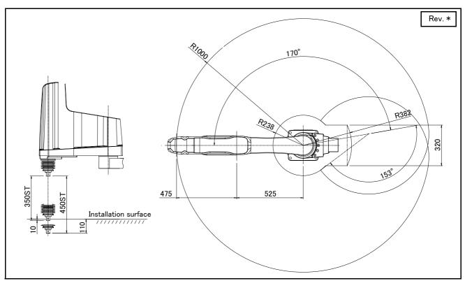
Fig.2-62 : Operating range diagram of RH-20FRH100xxC/M
