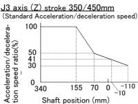
Note) The high acceleration-and-deceleration pattern of the type without illustration of the high acceleration-and-deceleration pattern is the same as the standard acceleration-anddeceleration pattern.
