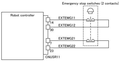
Fig.7-2 : How to wire emergency stop lines
