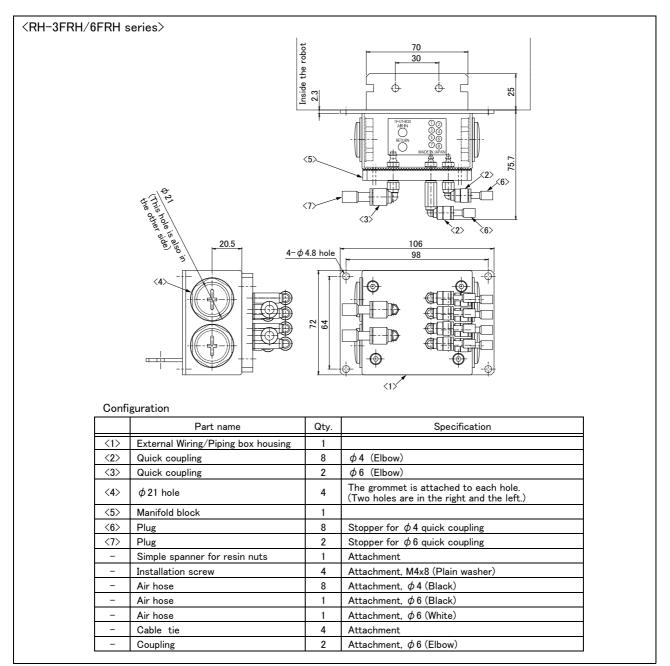
Fig.2-97 : Outline dimension and configurations (RH-3FRH/6FRH series)
