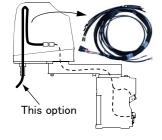
This set, consisting of air hoses and cables, is for feeding air hoses and hand input signal cables from the No. 2 arm through to the shaft tip.
