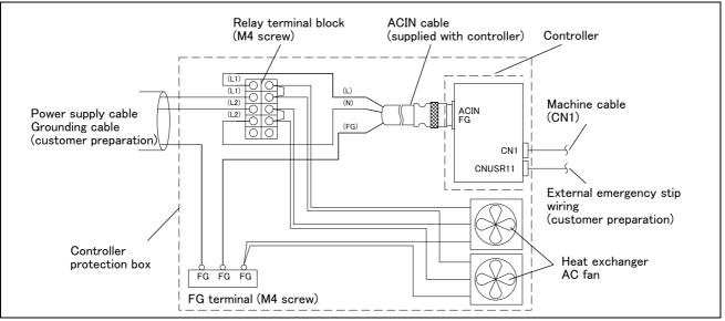
Fig.3-28 : Wiring system diagram
