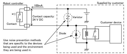
\*1) The actual internal robot controller circuit differs from the internal robot controller circuit in the figure.
