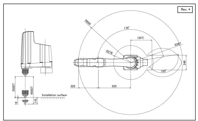
Fig.2-60 : Operating range diagram of RH-20FRH85xxC/M
