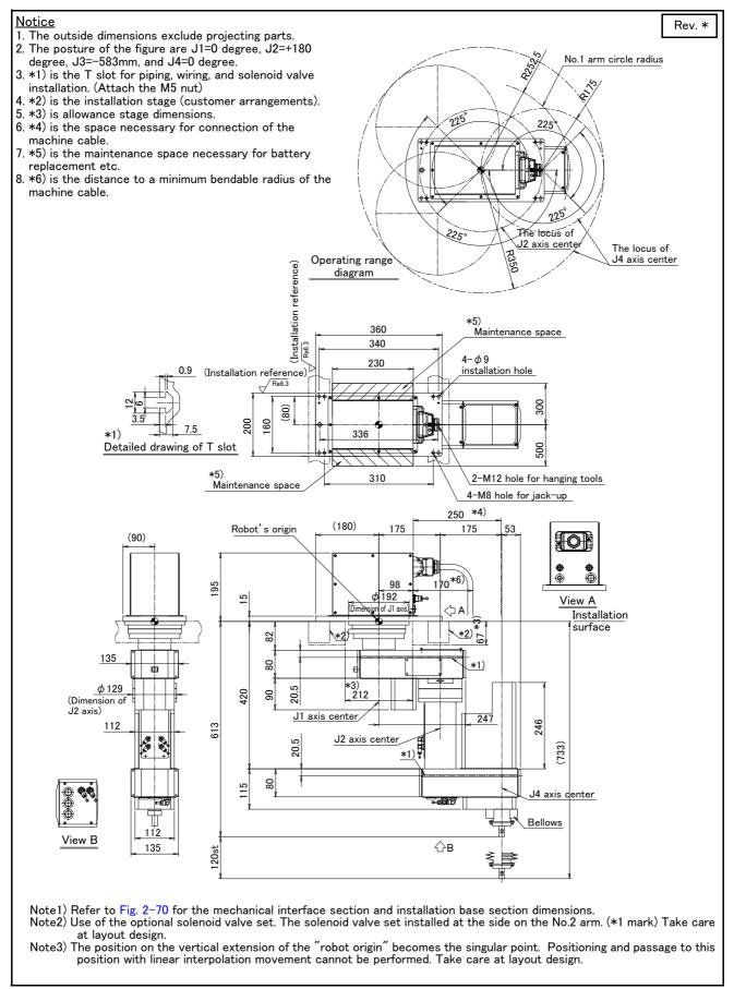
Fig.2-64 : Outside dimensions, Operating range diagram of RH-3FRHR series (Clean/waterproof specification)
