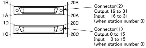
Fig.3-31 : Pin layout of connector
