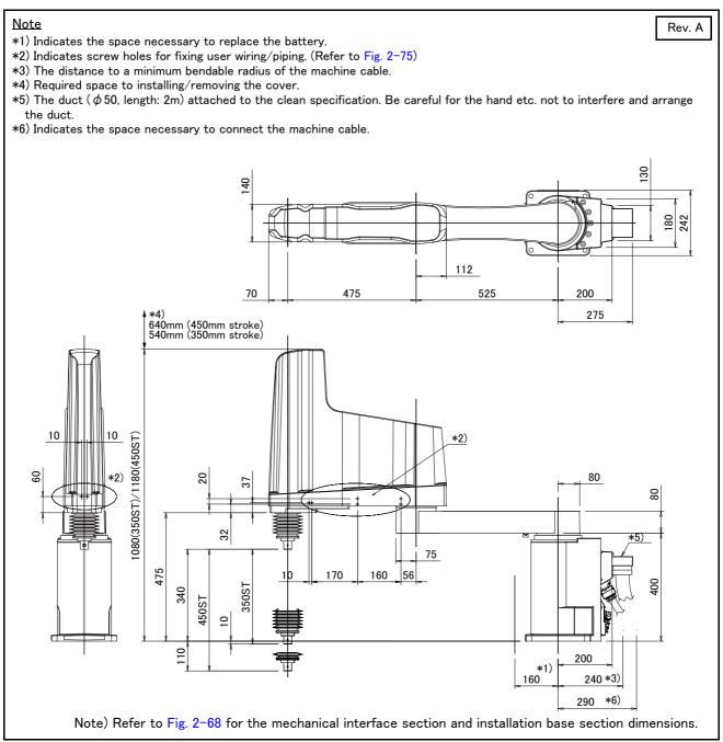
Fig.2-61 : Outside dimensions of RH-20FRH100xxC/M
