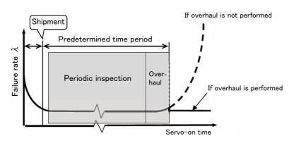
Fig.2-99 : Periodic inspection/overhaul periods
