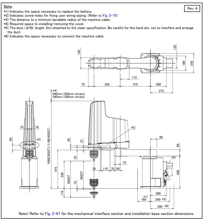
Fig.2-51 : Outside dimensions of RH-12FRH70xxC/M
