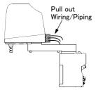
This is a very useful option when removing the air hoses and signal lines from the rear of the No. 2 arm, and pulling hand wiring and piping out to the robot's exterior. The joint for connects to the external hose is prepared, and the holes which fixes the signal cable to pull out with cable clamp are prepared. Optional hand output cables and hand input cables can be fixed here.
