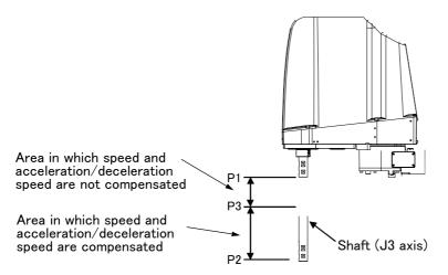
Fig.2-9 : Area in which acceleration/deceleration speed is compensated
