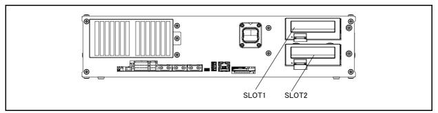
Fig.3-30 : Parallel I/O interface installation position
