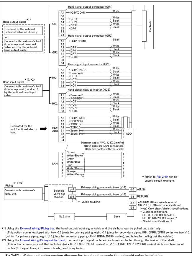
Fig.2-82 : Wiring and piping system diagram for hand and example the solenoid valve installation (RH-3FRH/6FRH/12FRH/20FRH series)
