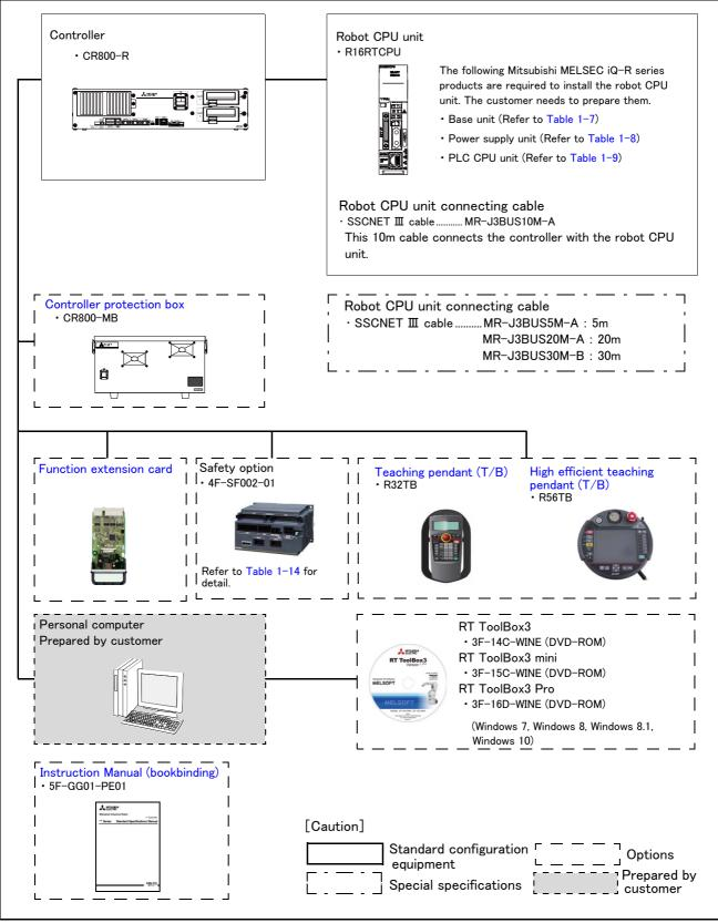
Fig.1-6 : Structural equipment (CR800-R)
