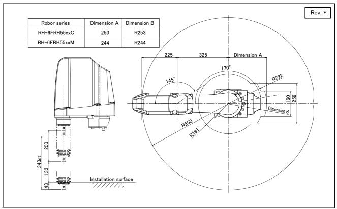
Fig.2-42 : Operating range diagram of RH-6FRH55xxC/M
