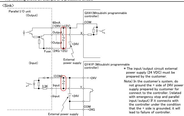
The following shows an example of a protective circuit.
