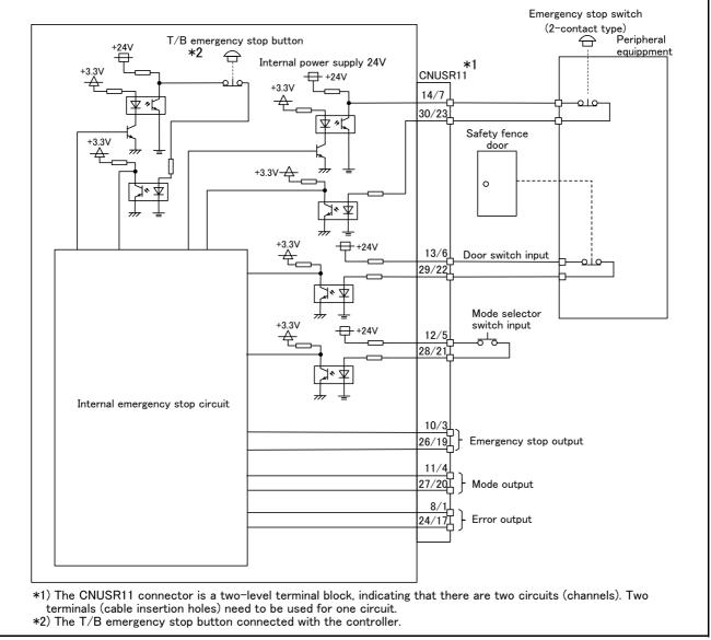
Fig.6-1 : Example of safety measures (wiring example 1)
