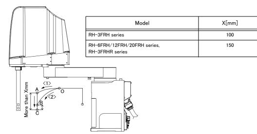
Fig.2-14 : Recommended path when positioning at the bottom edge of the Z axis
