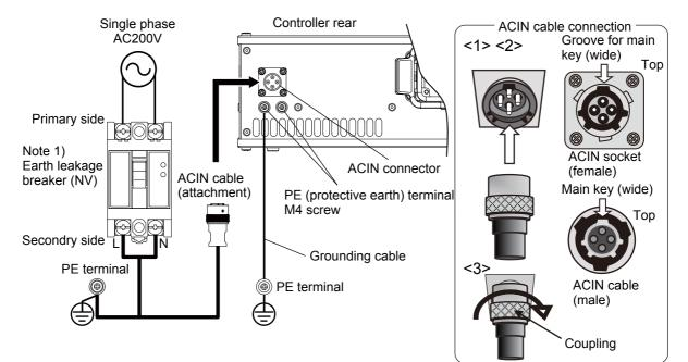
Note 1) Always use the terminal cover for the earth leakage breaker.
