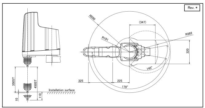
Fig.2-50 : Operating range diagram of RH-12FRH55xxC/M
