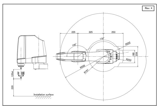
Fig.2-30 : Operating range diagram of RH-3FRH5512C
