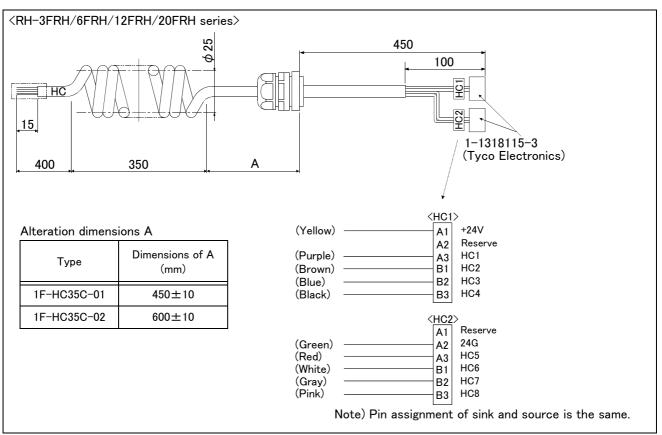
Fig.2-90 : Outside dimensional drawing and pin assignment (RH-3FRH/6FRH/12FRH/20FRH series)
