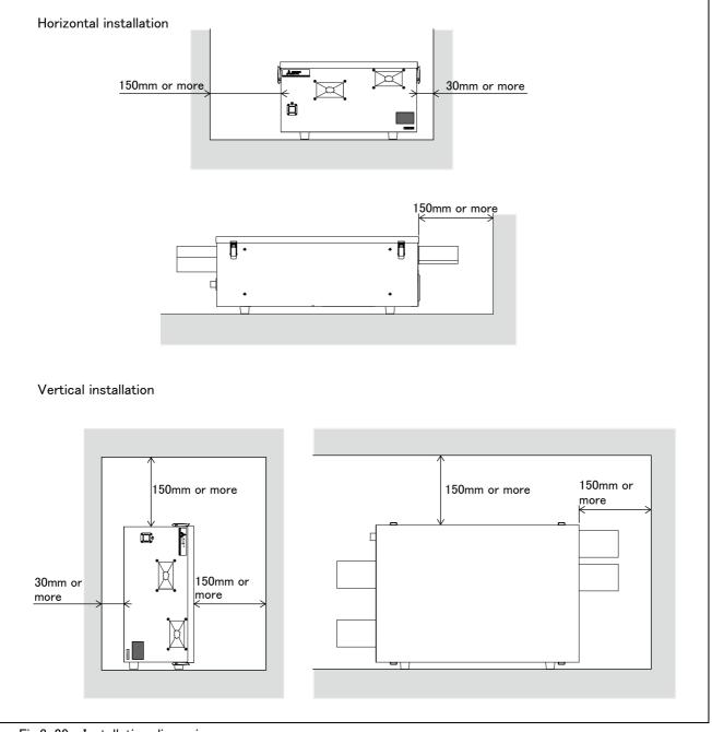
Fig.3-29 : Installation dimensions
