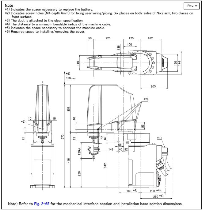
Fig.2-25 : Outside dimensions of RH-3FRH3512C
