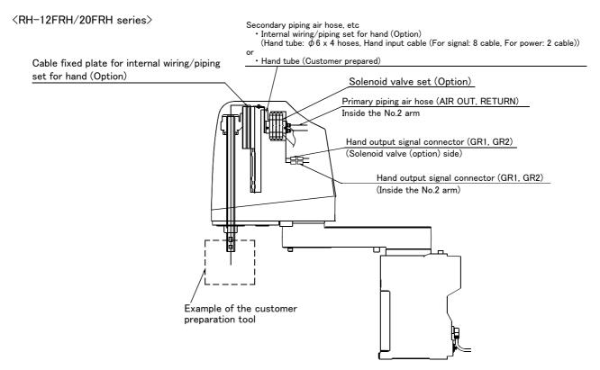
Fig.2-79 : Example of wiring and piping <1> (RH-12FRH/20FRH series)
