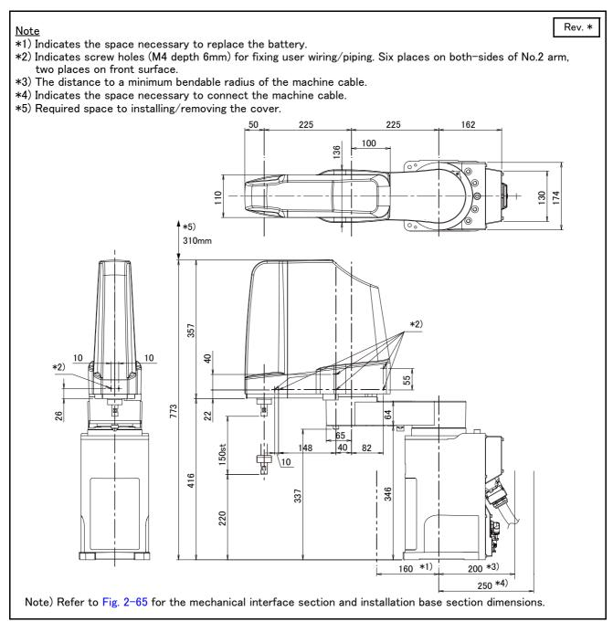
Fig.2-21 : Outside dimensions of RH-3FRH4515
