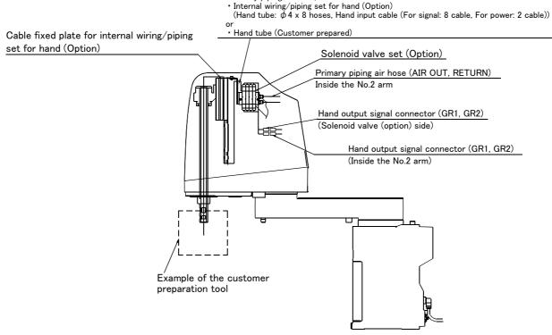
Fig.2-78 : Example of wiring and piping <1> (RH-6FRH series)
