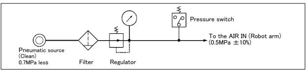
Fig.2-84 : Air supply circuit example for the hand
