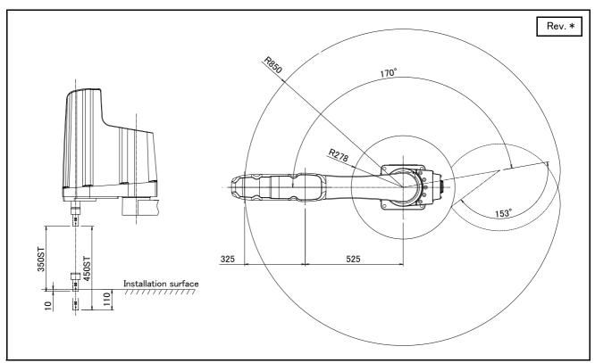
Fig.2-56 : Operating range diagram of RH-20FRH85xx
