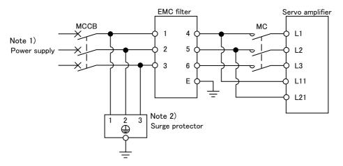
Note 1) For 1-phase 200V to 230VAC power supply, connect the power supply to L1, L2 and leave L3 open. There is no L3 for 1-phase 100 to 120 VAC power supply.
