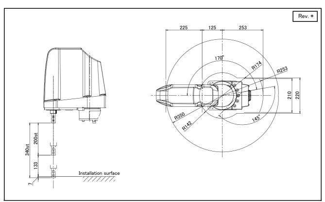
Fig.2-34 : Operating range diagram of RH-6FRH45xx
