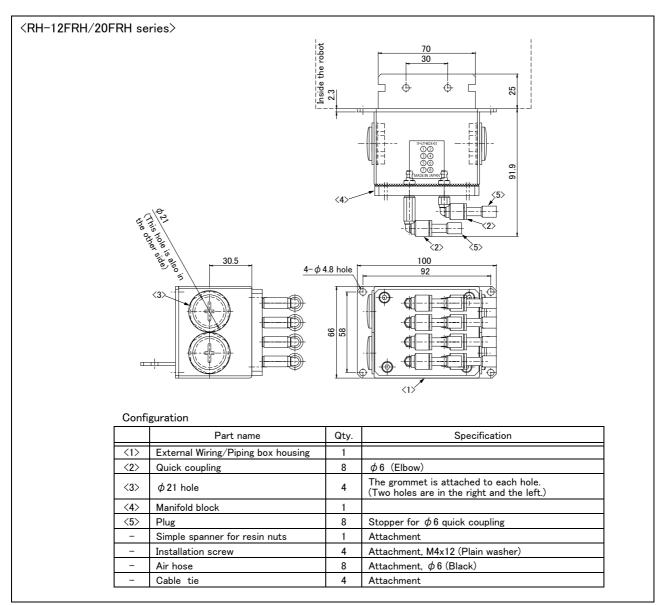
Fig.2-98 : Outline dimension and configurations (RH-12FRH/20FRH series)
