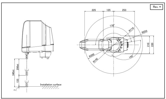
Fig.2-32 : Operating range diagram of RH-6FRH35xx
