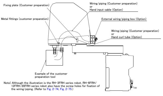
Fig.2-81 : Example of wiring and piping <2>
