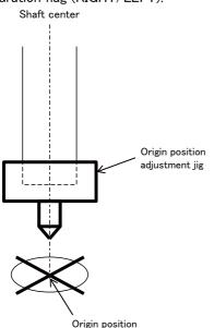
Fig.7-4 : Origin position adjustment
