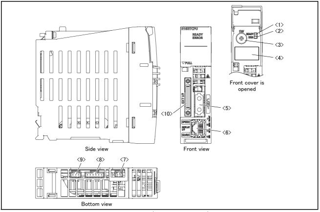
$\mathsf{Fig.3-2}$  : Names of each part of the robot CPU unit (CR800-R controller)
