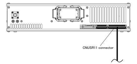
Fig.3-12 : Emergency stop cable and mode selector switch connection
