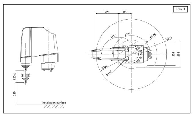
Fig.2-26 : Operating range diagram of RH-3FRH3512C
