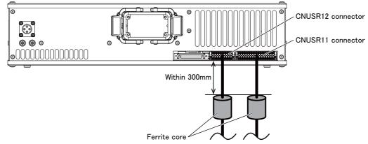
Fig.3-11: Installation position of ferrite cores
