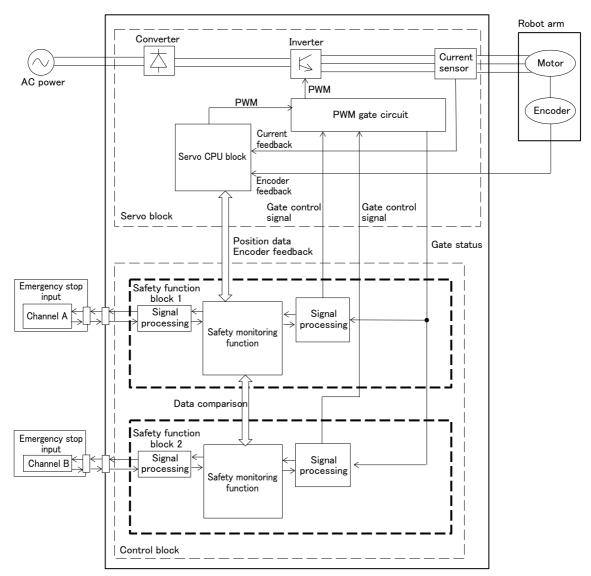
Fig.7-3 : Safety block diagram
