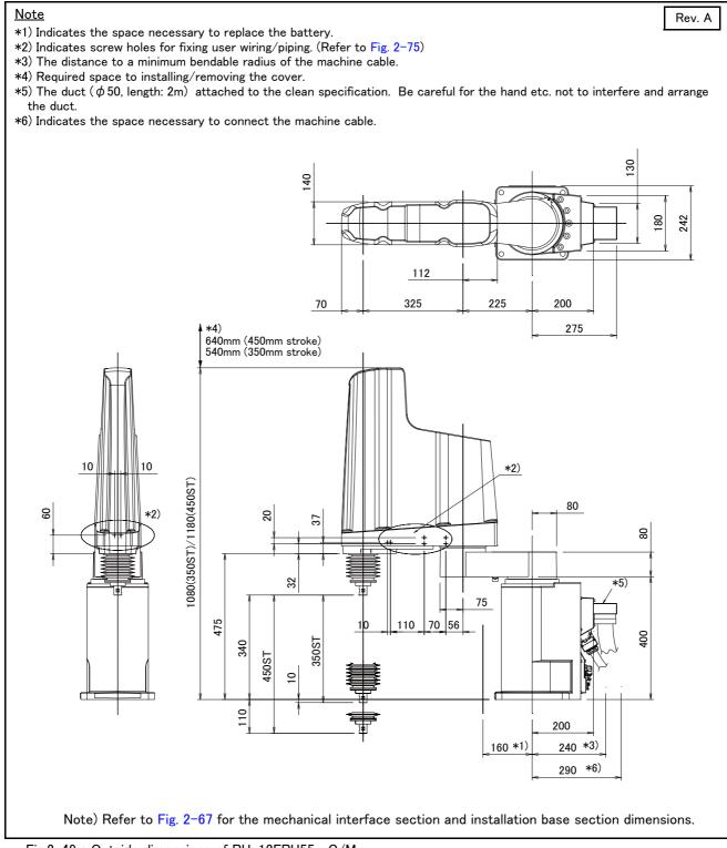
Fig.2-49 : Outside dimensions of RH-12FRH55xxC/M
