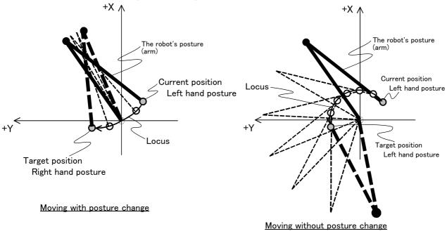
Fig.2-13 : Moving time by posture change (Conceptual Drawing)
