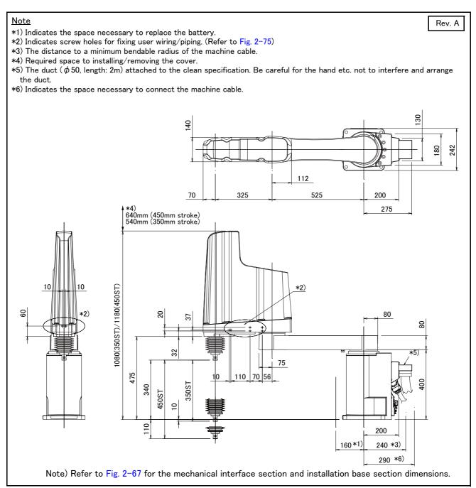
Fig.2-53 : Outside dimensions of RH-12FRH85xxC/M
