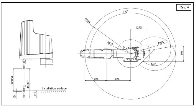
Fig.2-46 : Operating range diagram of RH-12FRH70xx
