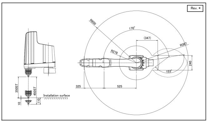
Fig.2-54 : Operating range diagram of RH-12FRH85xxC/M
