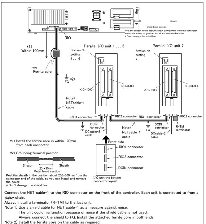
Recommended ferrite core: E04SR301334 (manufacture: SEIWA ELECTRIC MFG)
