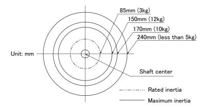
Fig.2-5 : Position of center of gravity for loads (for loads with comparatively small volume): RH-12FRH series
