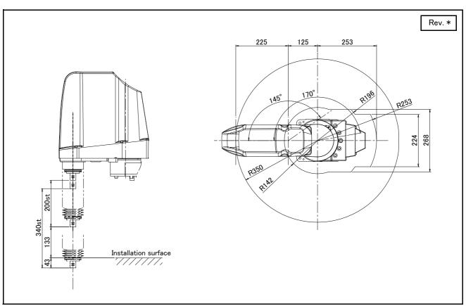
Fig.2-38 : Operating range diagram of RH-6FRH35xxC/M
