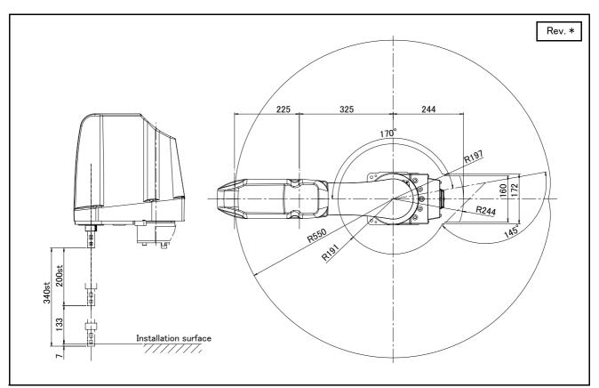
Fig.2-36 : Operating range diagram of RH-6FRH55xx
