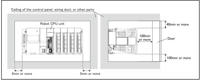
Fig.3-9 : Installation of robot CPU Unit
