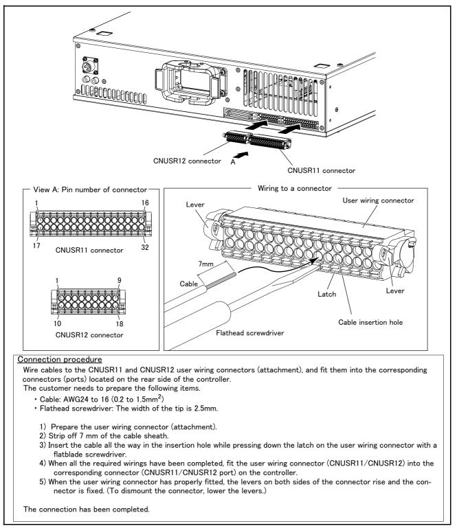
Fig.3-14 : Wiring method to the user wiring connector
