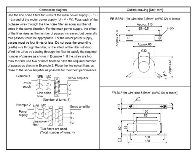
Fig.3-20 : Example of noise filter installation
