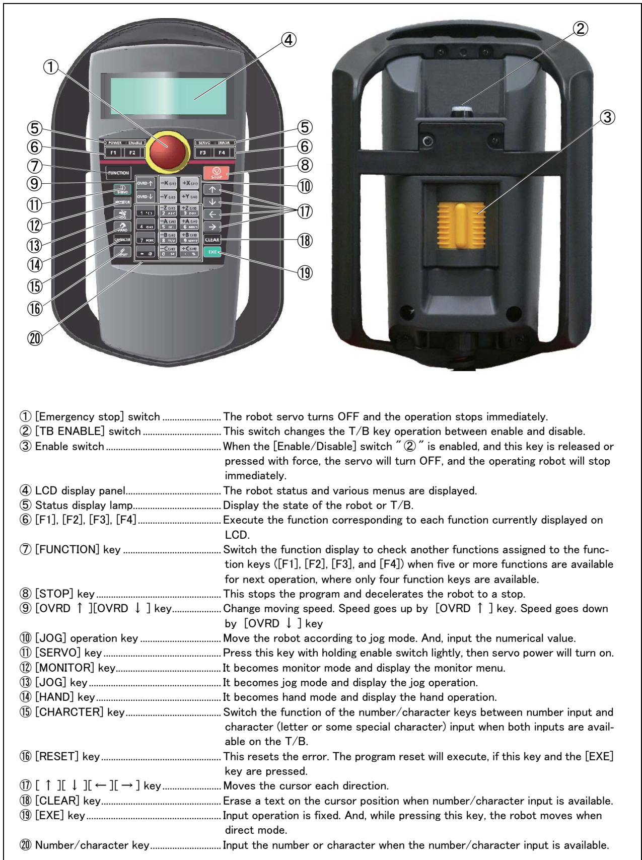
Fig.3-24 : Teaching pendant key layout and main functions
