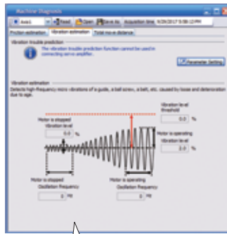
[Machine diagnosis function window on MR Configurator2]
