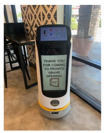
Pringle Robotics currently offers a number of different service robots including KettyBOT, which can simplify hosting, guiding, delivery, and advertising. Photo courtesy Pringle Robotics
