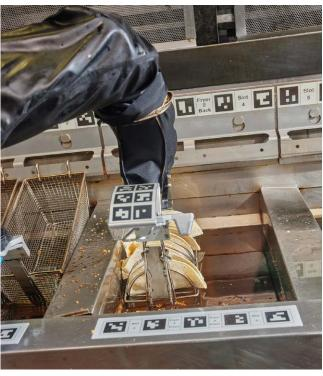
Flippy from Miso Robotics is the world's first-ever Al-powered robotic fry cook. With its incredible multitasking capabilities, Flippy can fry frozen ingredients and plate finished food with remarkable precision while keeping multiple recipes on the go. Photo courtesy Miso Robotics
