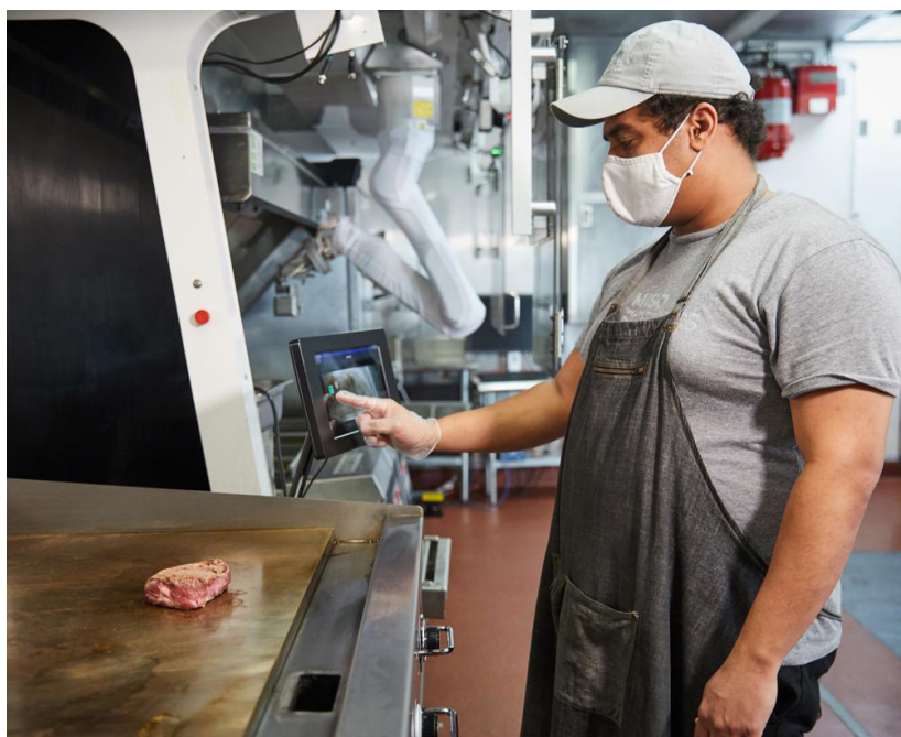
AI is already at play in catering spaces: Miso Robotics offers a software product that delivers AI-powered cooking with its Flippy robot. The CookRight platform uses cameras mounted above a grill along with a tablet computer. The cameras look down at the food being prepared and use a combination of computer vision, thermal detection, and AI to identify a cut of meat, its thickness, and cooking progress. Photo courtesy Miso Robotics
