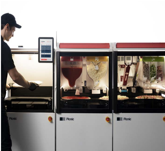
Picnic Works' Picnic Pizza Station is an automated, robotic back-of-house makeline that allows one person to make up to 100 consistent pizzas an hour, while reducing food waste to around 2%. Photo courtesy Picnic Works
