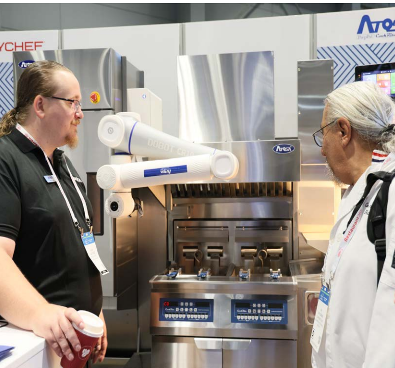
Artosa USA displayed its Intelligent French Fry Robotic Solution during the 2023 National Restaurant Association Show. The six-axis collaborative “co-bot” robot solution provides system adaptability during peak and non-peak times and allows the system to operate entirely manually when needed. Photo courtesy National Restaurant Association
