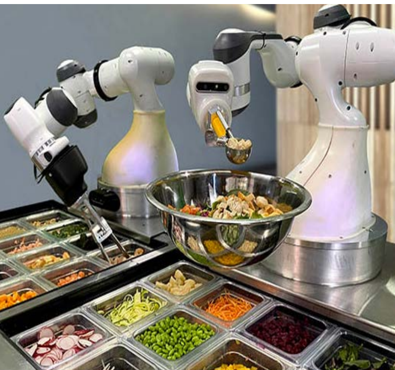
Dexai's robot dubbed "Alfred" can assemble dishes like salads and grain bowls. Photo courtesy Dexai
