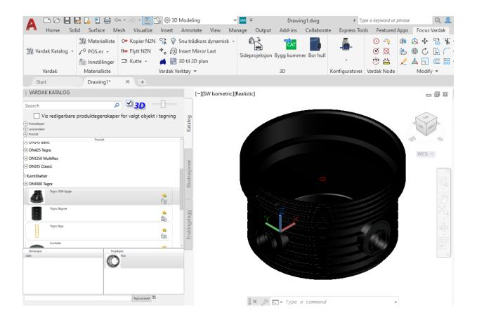
Each product on Focus Vardak has a unique name, product information and a node point to connect the parts correctly.
