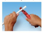
Out the pipe squarely at one of the '^' marks using recommended pipe cutters and ensure the pipe end is free from burrs (see page 12)
