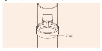
Figure 43: Use of Pipe Bracket Spacer
