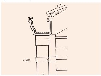
Figure 44: Application of Pipe Bracket Spacer
