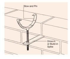
Figure 34: Installation of Rise and Fall Brackets
