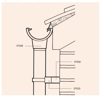
Figure 9: Use of Pipe Bracket Spacer
