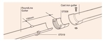
Figure 29: Connection to cast iron gutter
