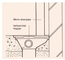
Figure 18: Connection to bottle gully
