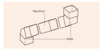
Figure 46: RoofLine shallow offset
