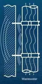
**Airborne sound** is the amount of noise from water passing through a pipe that can be heard if standing in the same room in which the pipe is installed **Structure-borne** sound is the amount of noise that can be heard from the pipe after the noise has permeated through pipe supports, brackets and walls
