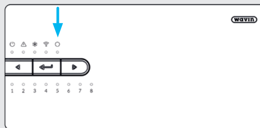
Enroll by navigating to the global channel. Wired outdoor sensor is enrolled automatically.
