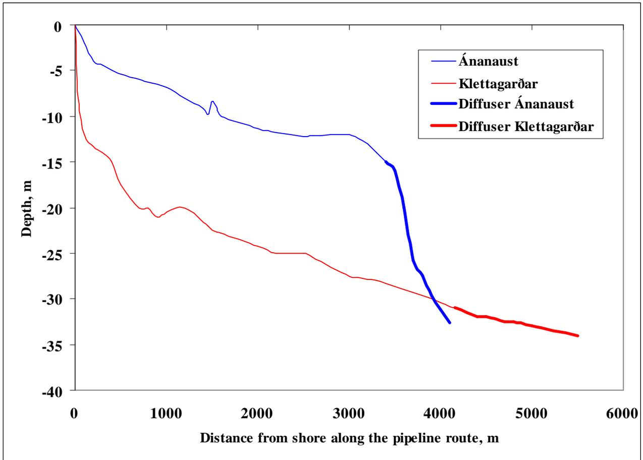
Figure 2 Depths along the route of the pipelines.
