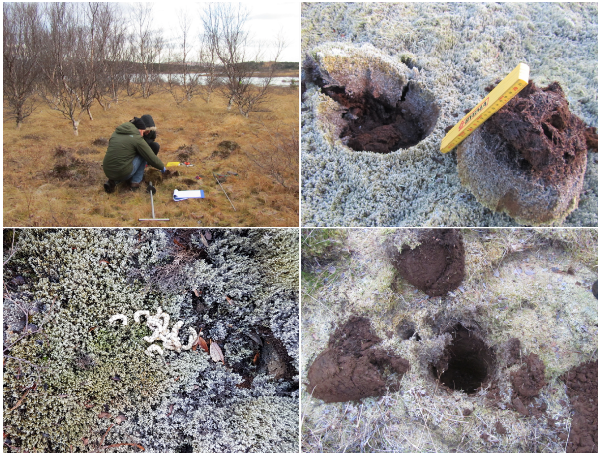
Figure 7: Images of soil sample collection in the Heiðmörk water catchment area in November 2018. (Top left) Soil sample collection in reworked area above well V-22. (Top right) Section of moss and soil. (Bottom left) Bird droppings in collected at Vatnsendakriki. (Bottom right) Hole dug for soil sample collection. Photographs courtesy of Veitur ohf.
