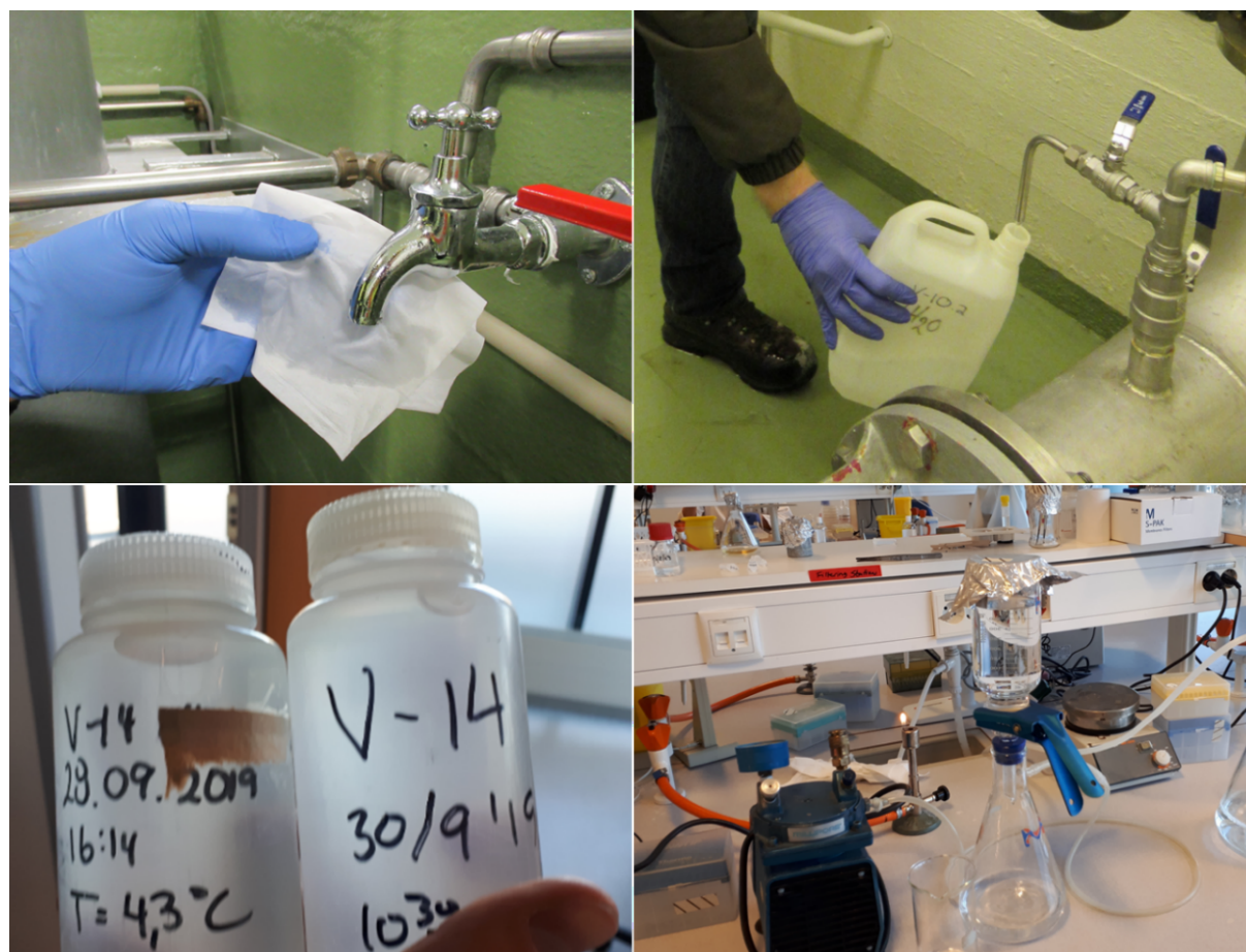
Figure 2: Images from well water sampling. Taps located after the well pumps were disinfected with 70% ethanol, flamed and rinsed by opening the tap for 5 minutes before collecting water samples for microbiome analysis (top left). Water samples for microbiome analysis were collected in sterile plastic containers directly from a pump outlet (top right). Water samples for cell counts were collected in sterile 200 ml plastic containers (bottom left). Water samples for microbiome analysis were filtered on 0.2 \mu\text{m} membrane filters and stored at -80^{\circ}\text{C} before DNA extraction (bottom right).
