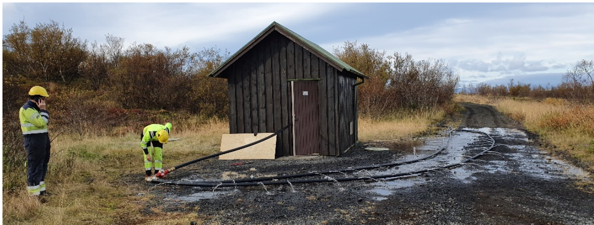
Figure 13: Distribution of well water around the pump house of well V14 during the simulated high precipitation event („Watering experiment“). Photograph courtesy of Veitur ohf.
