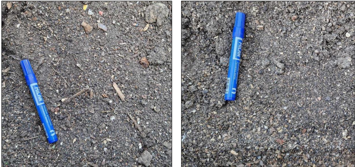
Figure 6. On the left is sand before screen change and on the right is sand after screen change, noticeably absent of >3\text{mm} material.
