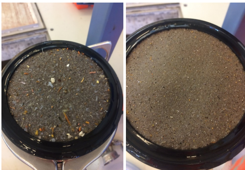
Figure 3 - Filters after sampling. 915 \mu m on the left and right 263 \mu m on the right.
