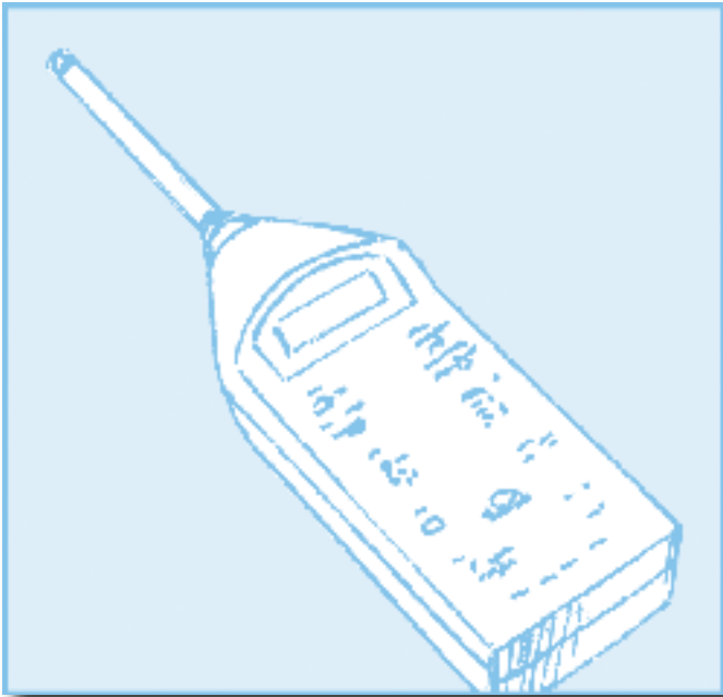
An integrating sound level meter averages noise levels over time.
