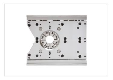
Depending on the capabilities of a 3rd party press used together with the Compact XL, rings can be crimped stroke prior or force prior. In case of force prior closing a constant compression rate can be achieved independently of material tolerances resulting in consistent reliable connecting solution and finally perfect application performance. Oetiker Service offers training and maintenance for its assembly solutions.
