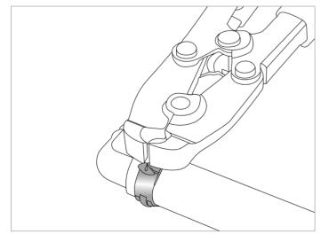
3. Cut through and remove clamp
