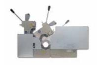
Oetiker Multi Crimp Rings should be assembled using the swaging tools developed for them. This ensures correct assembly and the best possible product performance. The compact, vertically opening design of the Two-Piece Swaging Tool for Multi Crimp Rings allows for separation of the two halves for optimum accessibility and automatic latching of the tool.
