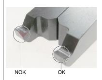
The followi "PrErr\_308: Crimping error CFM2 envelope curve 2"g criteria have led to the not OK evaluation: Second envelope curve (EO 2) right (Troubleshooting "PrErr\_308: Crimping error CFM2 envelope curve 2")
