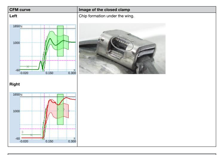
Slanting application; the right side is lower than the left side. Closure of the clamp on an oblique solid surface.
