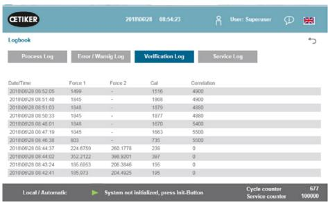
If a value is listed only for force 1, this is a tensioning force verification. The scaling factor is listed for the correlation factor to convert the PLC force sensor input signal into the closing force (see Section 9.5.2).
