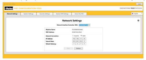
The IP address that is set is used both for the Ethernet TCP/IP and also for the Ethernet/IP (industrial communication).
