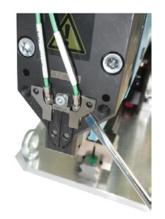
Before removing the crimping cut-off head, lay the force sensor cables (1) over the FAST 3000. This reduces the risk of inadvertently crushing the force sensor cables.
