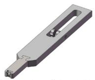
Fig. 32 Dismantled cut-off die and slide
