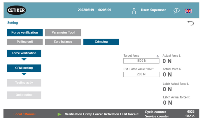
Fig. 57: Verification crimping force
