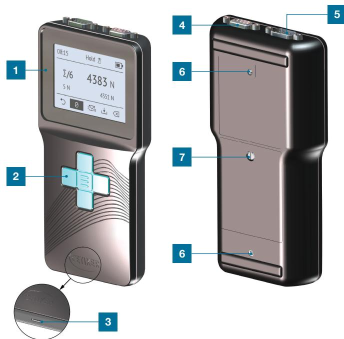
1 Display | 2 Control panel | 3 Charging port (USB-C) | 4 X5 interface fCAL 1 Closing Force Sensor (CFS) | 5 X3 interface PC / EPC 01 (RS232) | 6 2x M3 mounting threads for wall mounting | 7 Battery compartment
