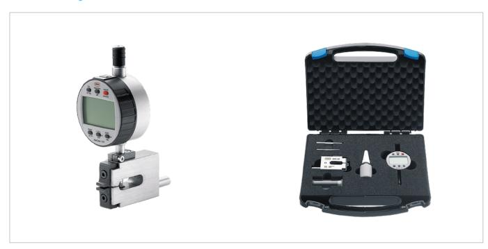
Mechanical alternative for closing force calibration
