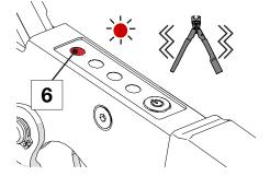
3. Release the handles of the pincer after the clamp is closed. The pincer is ready for next clamping operation.
