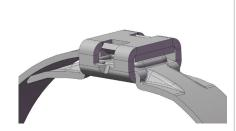
Cutting Remaining band is cut flush at housing. The residual band is ejected.
