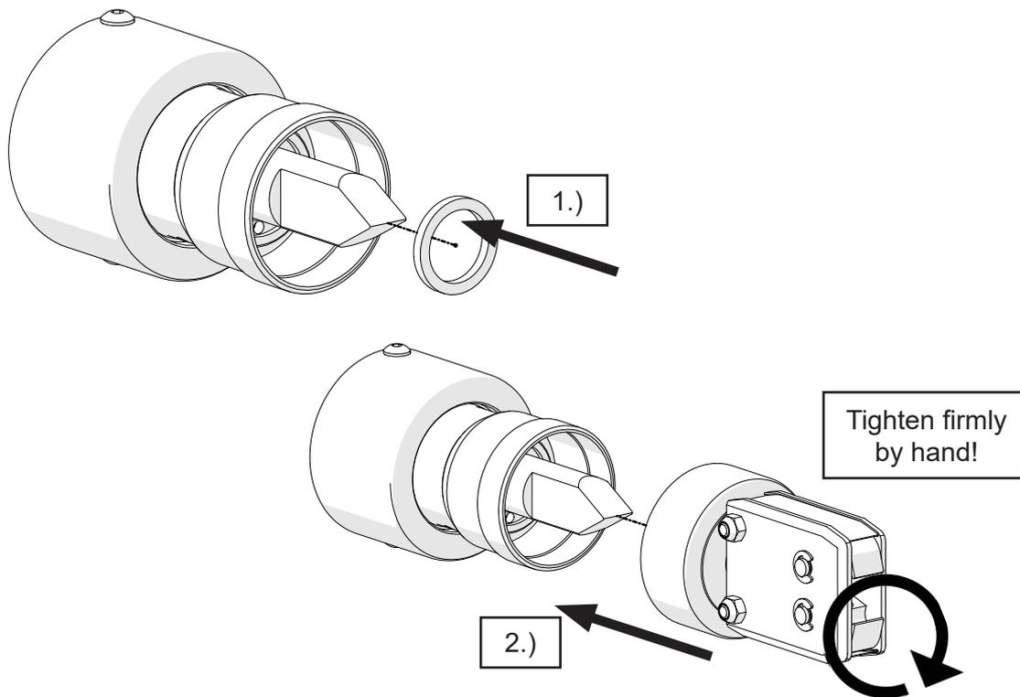
Fig. 36: Screw on the pincer head
