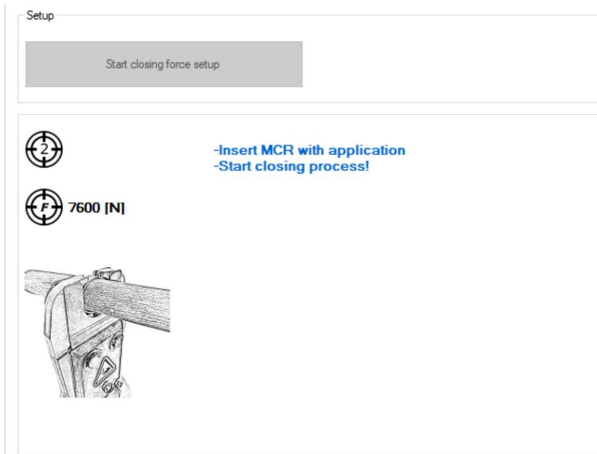
15. Repeat process until MCR closure incl. application (roundness MCR) is complete and within an acceptable roundness tolerance of  $\pm 0.2$  mm
