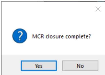
14. "No": Repeat the process, the thrust force now increases step by step by 1000 N:
