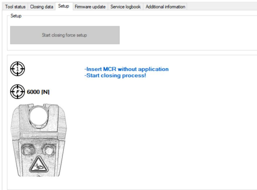
9. Repeat the procedure until MCR closure (MCR roundness) is complete and within an acceptable roundness tolerance of  $\pm 0.2$  mm
