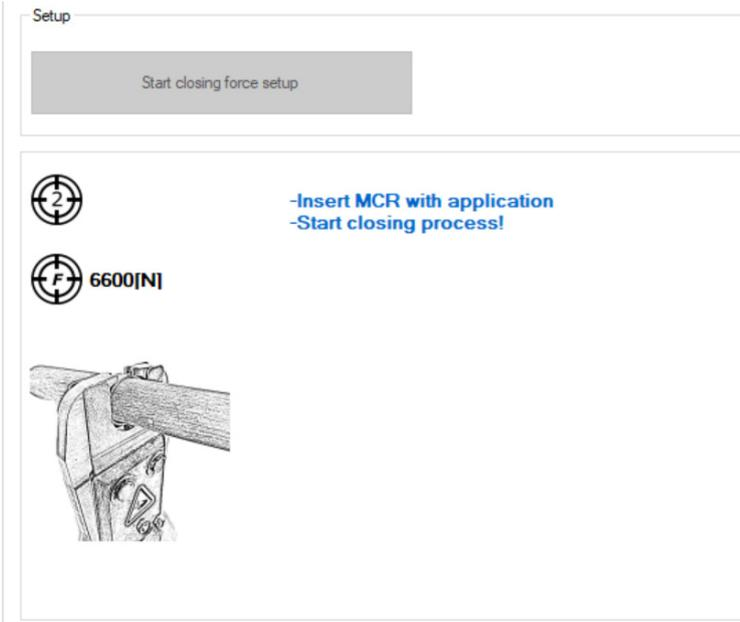
12. Check MCR for roundness, does the ring have the desired final external diameter and is it within  $\pm 0.2$  mm roundness?
