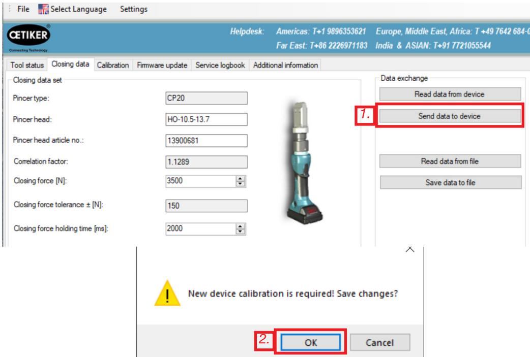
Fig. 32: Transfer closing force data
