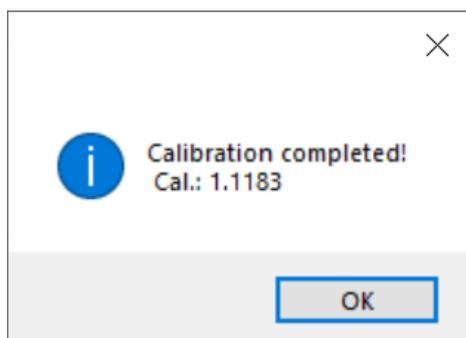
The "Calibration completed!" window now opens. This displays the calculated correlation factor (Cal.) (ratio between the thrust force of the plunger and the closing force of the pincer jaws) for information purposes
