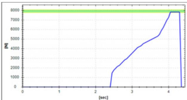
The force curve when closing with MCR or MCR and application should typically show a vertical force surge at the end. This indicates that the pincer jaws have been fully closed.
