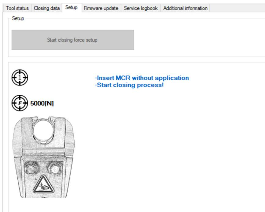
5. Insert MCR without application and perform a complete closing operation. This first closing process always starts with a minimum thrust of 5000 N.
