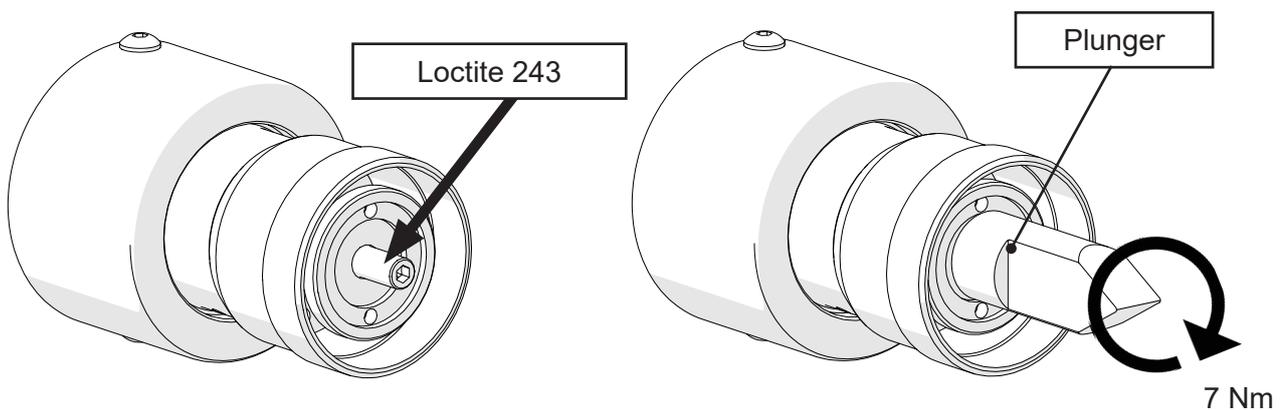
Fig. 35: Tighten the wedge
