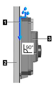
Fig. 6-11: Water drainage
