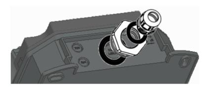
Fig. 7-17: Use of a reducing insert
