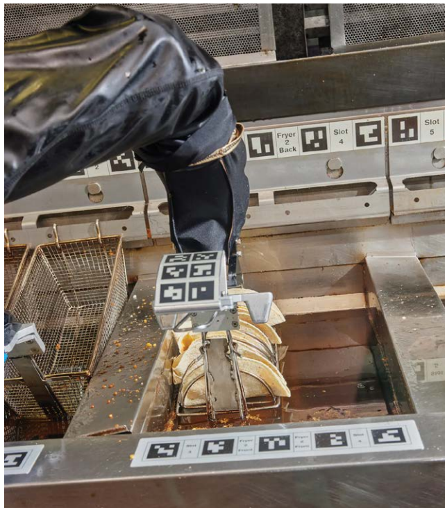
Flippy from Miso Robotics is the world's first-ever AI-powered robotic fry cook. With its incredible multitasking capabilities, Flippy can fry frozen ingredients and plate finished food with remarkable precision while keeping multiple recipes on the go. Photo courtesy Miso Robotics
