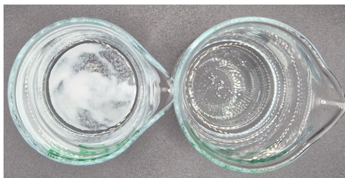
Figure 1 - left: standard MgO, right: Highly Active MgO in Citric Acid (2%)
